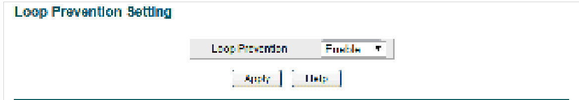
Figure 5-1 Configuring Loop Prevention
