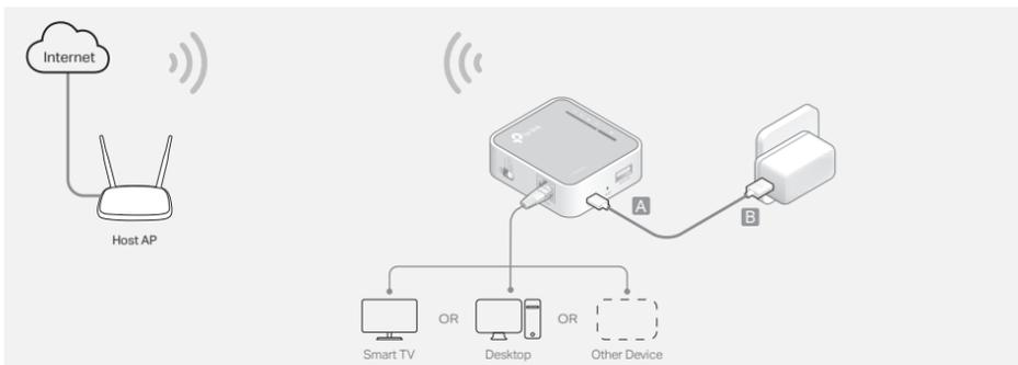
1. Switch the Mode Switch to AP/Rng Ext/Client and connect the hardware from Step A to B near your host AP.
