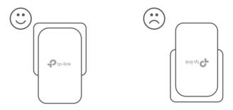
3. Plug the product directly into a wall socket instead of a power strip.
