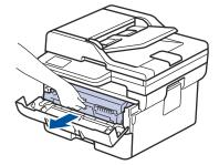
10. Push down the green lock lever and take the toner cartridge out of the drum unit.
