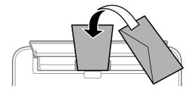
Load envelopes in the paper cassette with the flap facing up, and then slide the edge guides to the edges of the envelopes.
