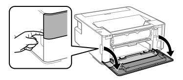
2. Lower the output switch lever.
