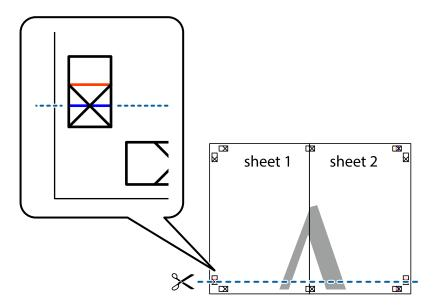
7. Place the edge of Sheet 1 and Sheet 2 on top of Sheet 3 and Sheet 4 and align the cross marks, and then temporarily tape them together from the back.
