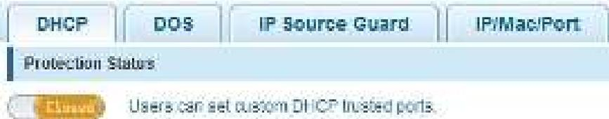
DHCP snooping is a security technology built into the operating system of a capable network switch that drops DHCP traffic determined to be unacceptable. The fundamental use for DHCP snooping is to prevent unauthorized (rogue) DHCP servers offering IP addresses to DHCP clients.
