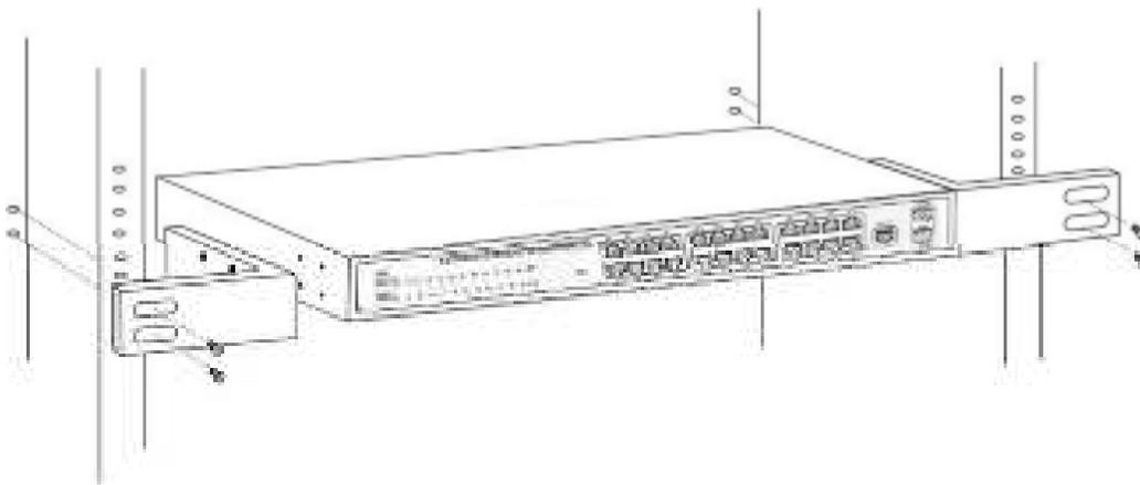
Figure 6 - Rack Installation
