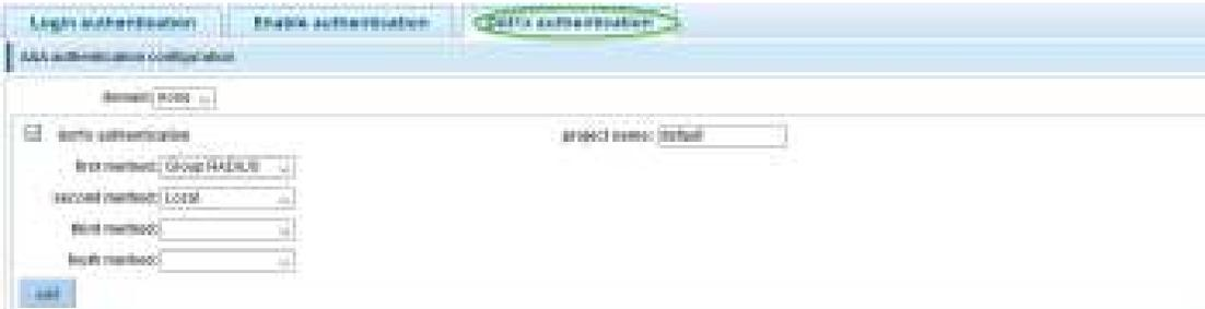
Note: If you activate this but have not configured any of the authentication methods (i.e., RADIUS) correctly, you will lose access to the Intellinet switch, and you may need to perform a hardware reset in order to re-gain access to the web admin interface. See section 2.4.1 Front Panel.
