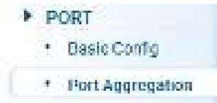
Port aggregation is a method of using multiple Ethernet ports in parallel to increase throughput beyond what a single connection could sustain and to provide redundancy in case one of the links should fail. As this is essentially a grouping of ports into one logical unit, we call them Link Aggregation Groups, or “LAG” for short.
