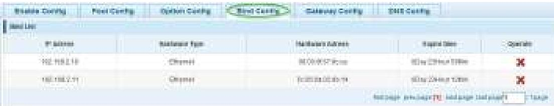
This page displays all clients that have obtained an IP address from the Intellinet switch. Click on
