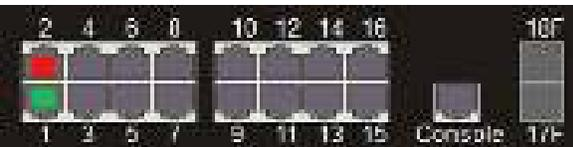
A green squares indicate the port link is up at Gigabit speeds (port 1 in the example above). A red squares indicates that a PoE device is connected (port 2). A gray squares indicate the port link is down.
