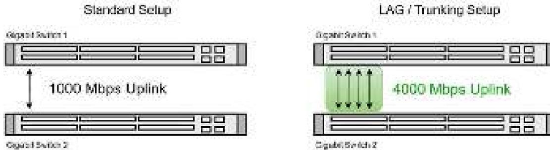
This page is used to set up LAGs. Create up to eight different LAGs; each can have up to eight member ports. Each LAG can be given a custom name, and you must select the ports for the LAG. The example below shows an LAG group set up with four member ports.
