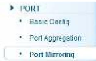
Port mirroring is the ability of a network switch to send a copy of network packets seen on a switch port or ports to a network-monitoring device connected to another switch port (i.e., a computer equipped with a packet sniffer utility). The Intellinet 16-Port Gigabit Ethernet PoE+ Web-Managed Switch provides up to four groups for port-mirroring settings.
