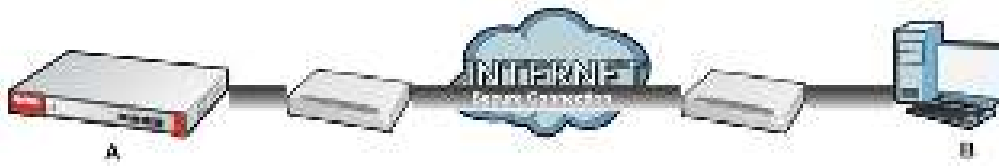
Figure 400 SSH Communication Over the WAN Example
