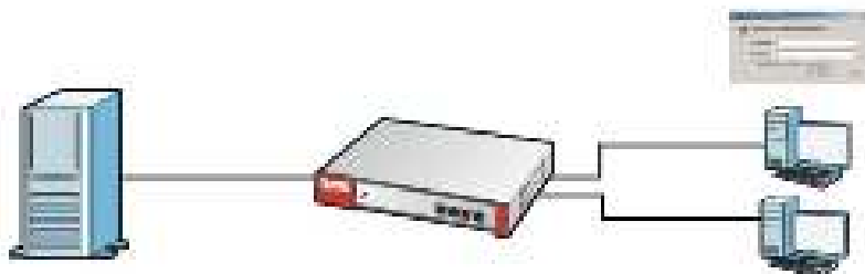
Figure 342 RADIUS Server Network Example
