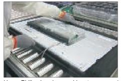
Use a Philips-head screwdriver to remove 4pcs screws for unlocking the bracket with panel module.
