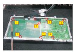
Remove the power board board and interface
