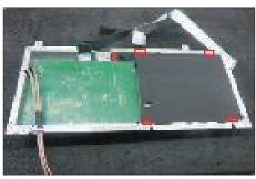
Use a Philips-head screwdriver to remove 7pcs
