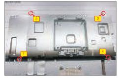
Move up the bracket, then disconnect the LVDS cables away from the connectors of the panel.
