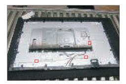
S12 Disconnect the panel lamp cables from the two connectors of the panel module, then tear off 1pcs aluminum foil as the picture below shown.
