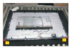
Disconnect the LED cable from the connector of the interface board, then release the LED cable by tearing off the 2pcs tapes.
