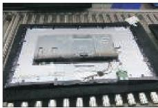
Tear off 1pcs acetate. Use a Philips-head screwdriver to remove one screw for unlocking the USB board, then disconnect the USB FFC cable and remove away the USB board.
