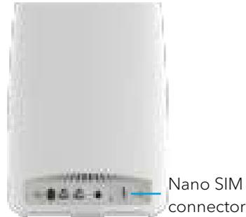
**IMPORTANT:** Make sure that the 4G LTE Orbi is powered off before inserting a nano SIM card.
