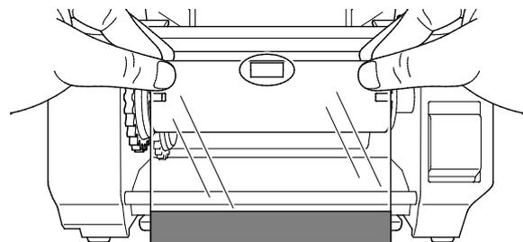
9. Using the Ribbon Rewind Gear, rotate the Ribbon Rewind Hub until the ribbon plastic leader is thoroughly wound and the black section of the ribbon covers the Print Head.
