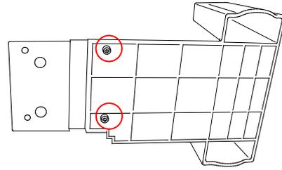
2. Attach the extended plate to the bottom of the printer.
