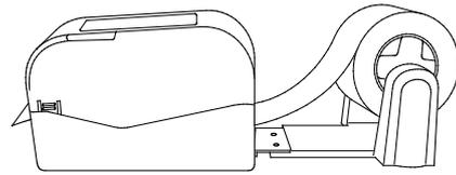
5. Open the Roll Compartment Cover. Slide the Roll Guides outwards, and then align the paper width with the Roll Guides. Push down the lock switch to lock the Roll Guide.
