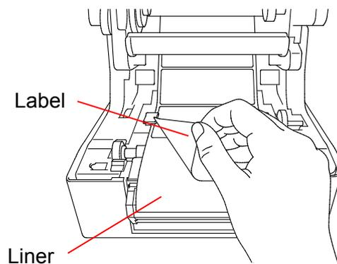
6. Open the Label Peeler Cover. Feed the liner into Label Peeler Cover Slot.
