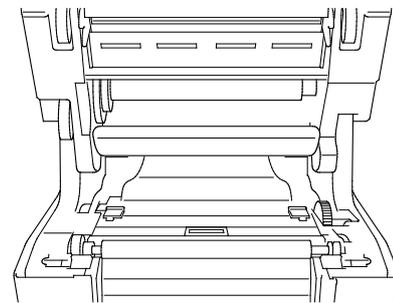
6. Insert the Ribbon Spindle into the ribbon.
