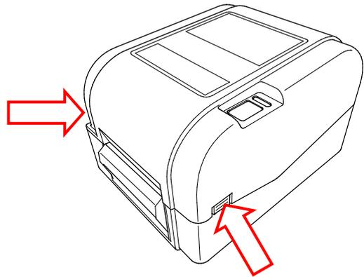
4. Push the Print Head Release Button to open the Print Head mechanism and feed the media through the media sensor. Adjust the Media Guide Tips to fit the label width.
