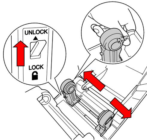
3. Insert the paper roll with the labels facing up, as shown in the illustration.
