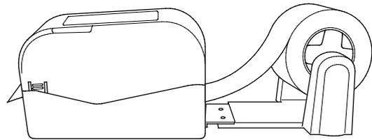
3. Insert a 3" (76.2 mm) Label Spindle into a paper roll. Then, install it on the External Paper Roll Mount.
