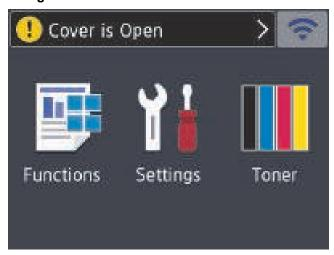
The warning icon appears when there is an error or maintenance message; press to view it, and then press to return to Ready Mode.
