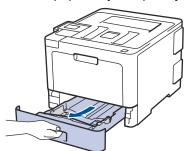
3. Make sure the jammed paper does not remain inside the machine.
