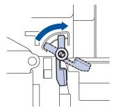
8. Using the green handle, push the drum unit back into the machine until it locks in place.
