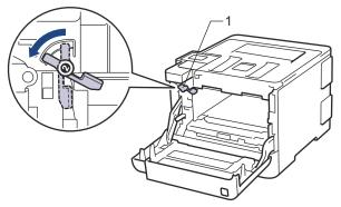
10. Gently slide the drum unit into the machine until it stops at the green lock lever.
