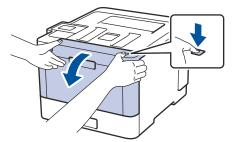
3. Hold the drum unit's green handle. Pull the drum unit out of the machine until it stops.
