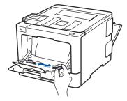
5. Load paper with the printing surface face up in the MP tray.
