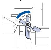
10. Using the green handle, push the drum unit back into the machine until it locks in place.
