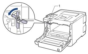
8. Gently slide the drum unit into the machine until it stops at the green lock lever.
