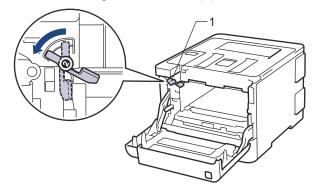
15. Gently slide the drum unit into the machine until it stops at the green lock lever.
