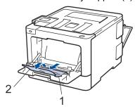
5. Slide the MP tray paper guides to fit the width of the envelopes that you are using.
