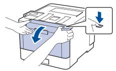
6. Hold the drum unit's green handle. Pull the drum unit out of the machine until it stops.
