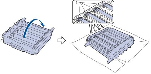
9. Use the numbered markers next to the drum roller to find the mark. For example, a cyan dot in column 2 on the check sheet would mean that there is a mark in the "2" region of the cyan drum.
