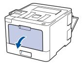
4. Pull out the MP tray support (1) and unfold the flap (2).
