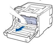
4. Hold the handle of the toner cartridge and gently push it away from you to unlock it. Pull it up and out of the drum unit. Repeat this for all toner cartridges.
