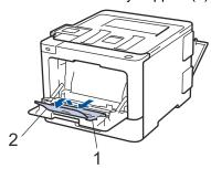
4. Slide the MP tray paper guides to fit the width of the paper that you are using. If the paper guide on the right side has a lever, press it and slide the paper guide.
