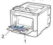
4. Slide the MP tray paper guides to fit the width of the paper you are using. If the paper guide on the right side has a lever, press it and slide the paper guide.
