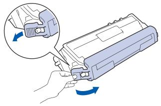
8. Insert the toner cartridge into the drum unit and gently pull it toward you until you hear it lock into place. Make sure that you match the toner cartridge colour to the same colour label on the drum unit. Repeat this for all toner cartridges.
