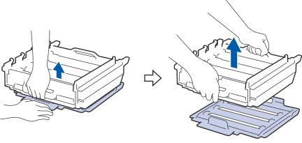
7. Hold the handle of the toner cartridge and gently push it away from you to unlock it. Pull it up and out of the drum unit. Repeat this for all toner cartridges.
