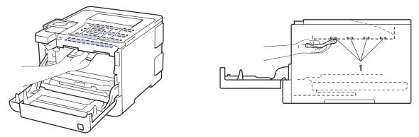
6. Make sure the green lock lever (1) is in the release position, as shown in the illustration.
