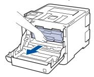
3. Hold the handle of the toner cartridge and gently push it away from you to unlock it. Pull it up and out of the drum unit. Repeat this for all toner cartridges.
