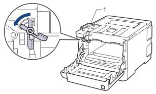
16. Gently slide the drum unit into the machine until it stops at the green lock lever.
