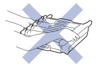
5. Hold the green handle of the belt unit with both hands and lift the belt unit up, then pull it out.
