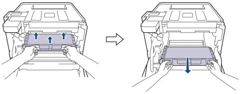
6. Unpack the new belt unit and install the new belt unit in the machine. Make sure the belt unit is level and fits firmly into place.
