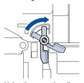
9. Using the green handle, push the drum unit back into the machine until it locks in place.
