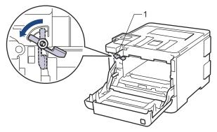
6. Gently slide the drum unit into the machine until it stops at the green lock lever.
