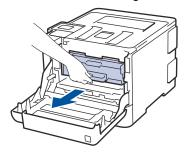
3. Turn the green lock lever (1) counterclockwise until it locks in the release position. Holding the green handles of the drum unit, lift the front of the drum unit and remove it from the machine.
