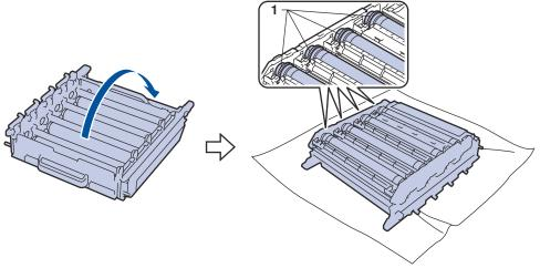
10. Use the numbered markers next to the drum roller to find the mark. For example, a cyan dot in column 2 on the check sheet would mean that there is a mark in the "2" region of the cyan drum.
