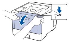
5. Hold the drum unit's green handle. Pull the drum unit out of the machine until it stops.
