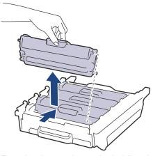
8. Turn the drum unit over by holding the green handles. Make sure that the drum unit gears (1) are on the left side.
