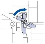
17. Using the green handle, push the drum unit back into the machine until it locks in place.
