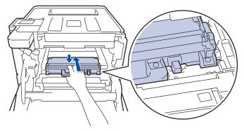
9. Slide the belt unit back into the machine. Make sure the belt unit is level and fits firmly into place.
