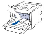
4. Turn the green lock lever (1) counterclockwise until it locks in the release position. Holding the green handles of the drum unit, lift the front of the drum unit and remove it from the machine.
