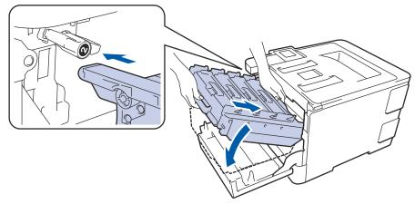
11. Turn the green lock lever clockwise to the lock position.
