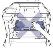
5. Make sure the green lock lever (1) is in the release position, as shown in the illustration.
