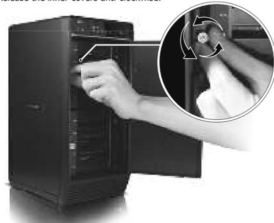
4. Install the HDDs from up to down.
