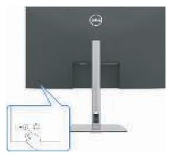
S2 Unplug external cables(power cable and video cable) from the monitor.
