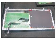
Use a Philips-head screwdriver to remove 8pcs
