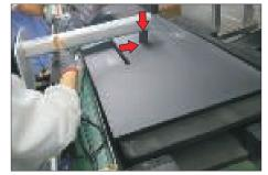
Use a Philips-head screwdriver to remove 4pcs screws for unlocking mechanisms.
