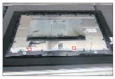
Take away the middle bezel, and put it on a fixture, then tear off the mylar tape for releasing the LED board.
