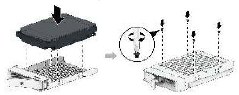
• For 2.5" drives: Place the drive in the drive tray. Turn the tray upside down and tighten screws into the four spots indicated below to secure the drive.
