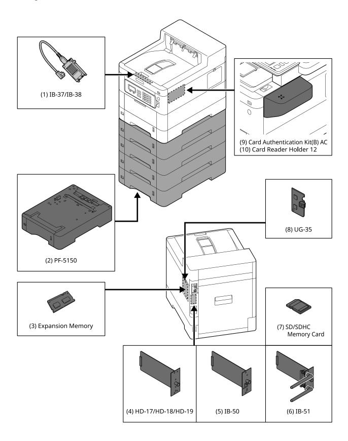
1 IB-37/IB-38 <Wireless network interface (USB: 5GHz/2.4GHz)>
