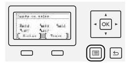
Displays the direction of arrow keys that are useable on the displayed screen.
