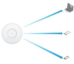
MU-MIMO with 2x2 and 1x1 clients: Each client radio of the the UniFi XG AP communicates with one 2x2 client and two 1x1 clients at a time.
