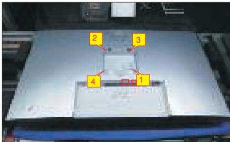
Wedge your fingers between rear cover and the middle bezel on the corners of the top side of the monitor to release the rear cover, then use one hand to press the middle bezel, the other hand to pull up carefully the rear cover in order of arrow preference for unlocking mechanisms of rear cover.
