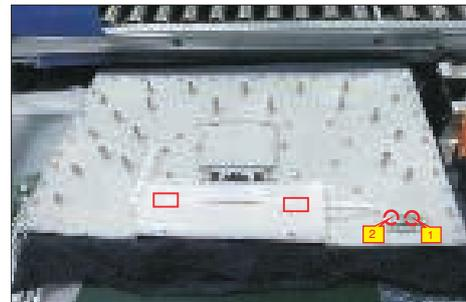
Move the assembled rear cover close to the panel unit, then connect the joystick key cable to the connector of interface board. Put down the rear cover and push the rear cover on the positions marked as the picture below shown for mechanisms engagement.
