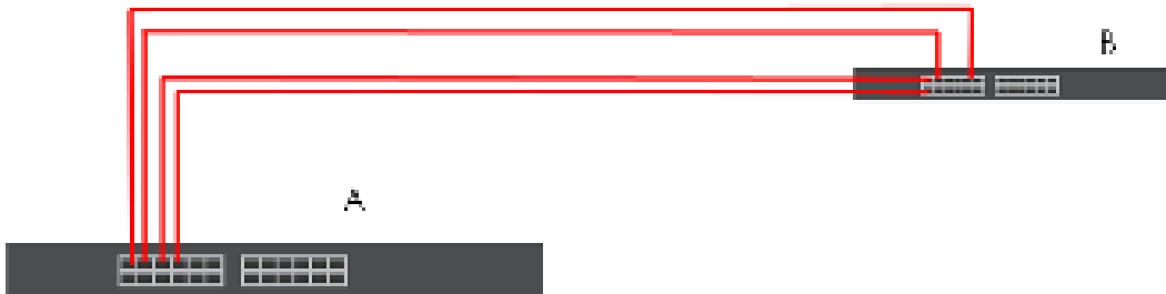
Figure 132 Trunking Example - Physical Connections
