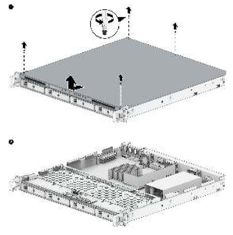
**Note:** When you remove the top cover, sensitive internal components are exposed. Avoid touching anything other than the memory assembly when removing or adding memory.
