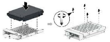
• For 2.5" drives: Place the drive in the drive tray. Flip the tray over and tighten screws into the four spots indicated below to secure the drive in place.
