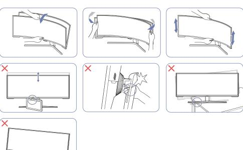
• Hold the bezel at both side edges and adjust the monitor angle until the screen becomes level. (Be
