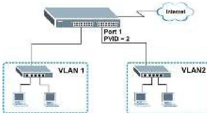
Figure 39 Initial Setup Network Example: Port VID
