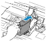
**2.** Close the ink cartridge locking cover to secure the FINE cartridge.
