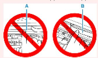
If you soil or scratch this part by touching it with paper or your hand, it could damage the printer.
