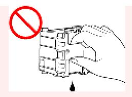
• Put the used one immediately into the plastic bag that came with the new maintenance cartridge and seal the bag by tying the opening tightly to prevent the ink from leaking.
