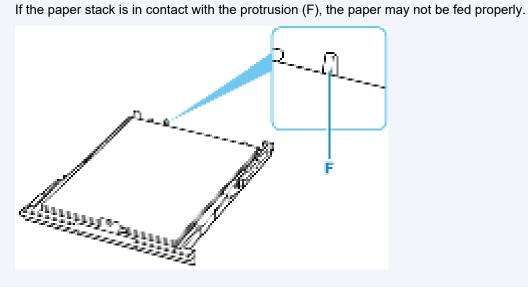
**5.** Move the front paper guide and adjust the guide to edge of the paper stack.
