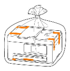
**7.** Attach the protective material to the printer when packing the printer in the box.
