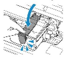
Make sure FINE cartridge holder motion is not impeded by protective material, jammed paper, etc.
