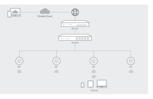
• Before you start, be sure to power up and connect your devices according to the topology figure. • A DHCP server (typically a router with DHCP function enabled) is required to assign IP addresses to the APs and clients in your local network.
