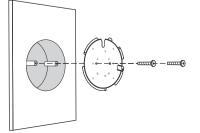
Route the cables through the square cable hole on the mounting bracket, and secure the mounting bracket to the junction box using screws. Then follow Step 4 and Step 5 of Option 2 to complete the installation.
