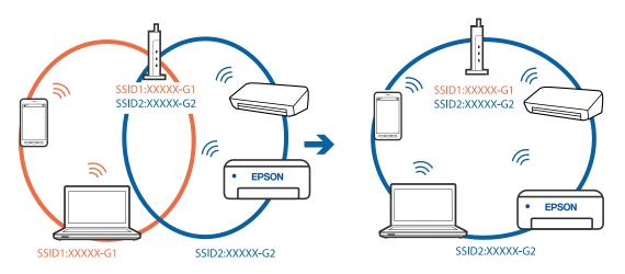
□ Example of connecting to SSIDs with a different frequency range
