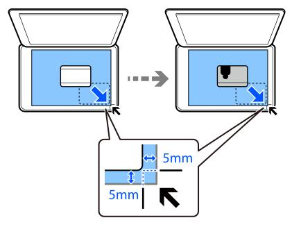
8. Place the back of the original face down, slide it to the corner mark, and then press the  $\triangle$  button.
