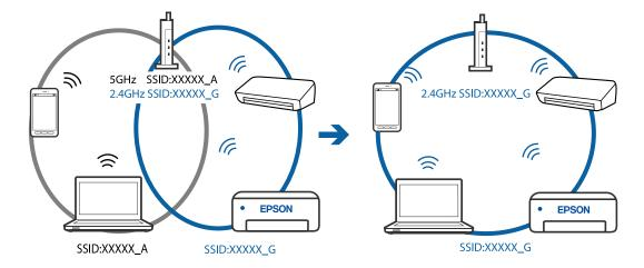
**L** Example of connecting to SSIDs with a different frequency range
