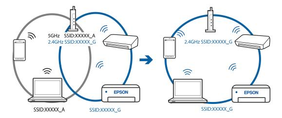
**L** Example of connecting to SSIDs with a different frequency range
