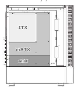
CPU cooler max height: 166mm
