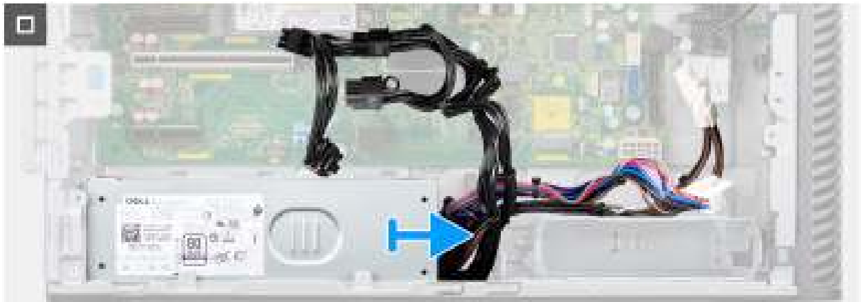
Figure 49. Removing the 1000W power-supply unit
