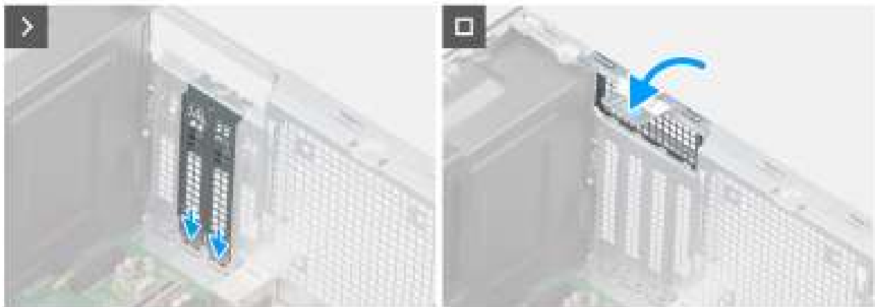
Figure 42. Removing the powered GPU
