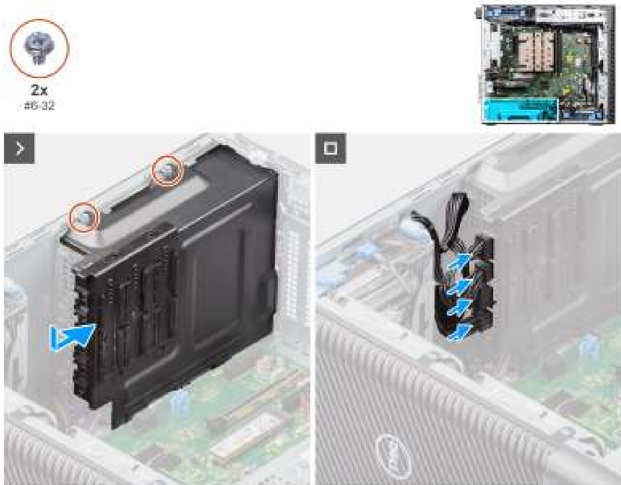
Figure 47. Installing the power-supply unit cover
