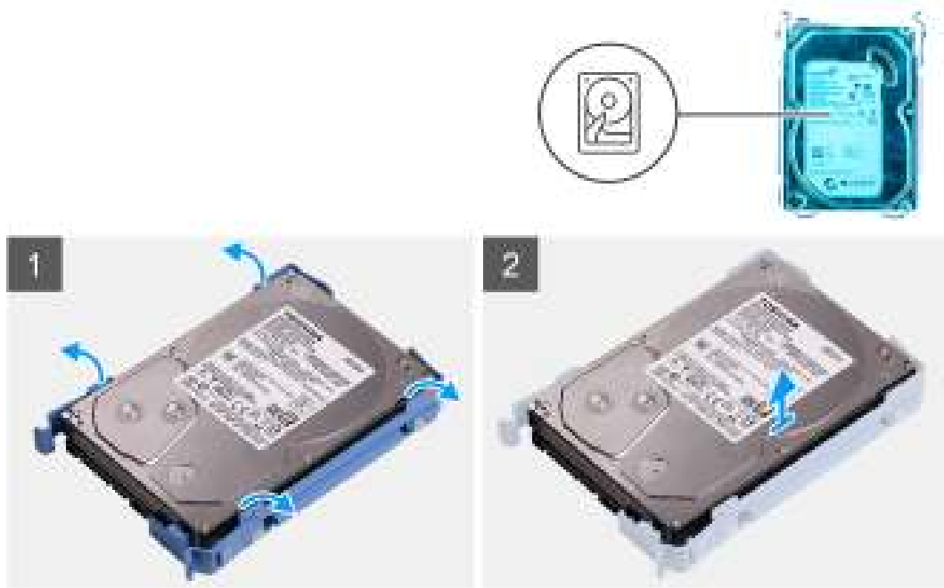
Figure 18. Removing the 3.5-inch hard-disk drive bracket
