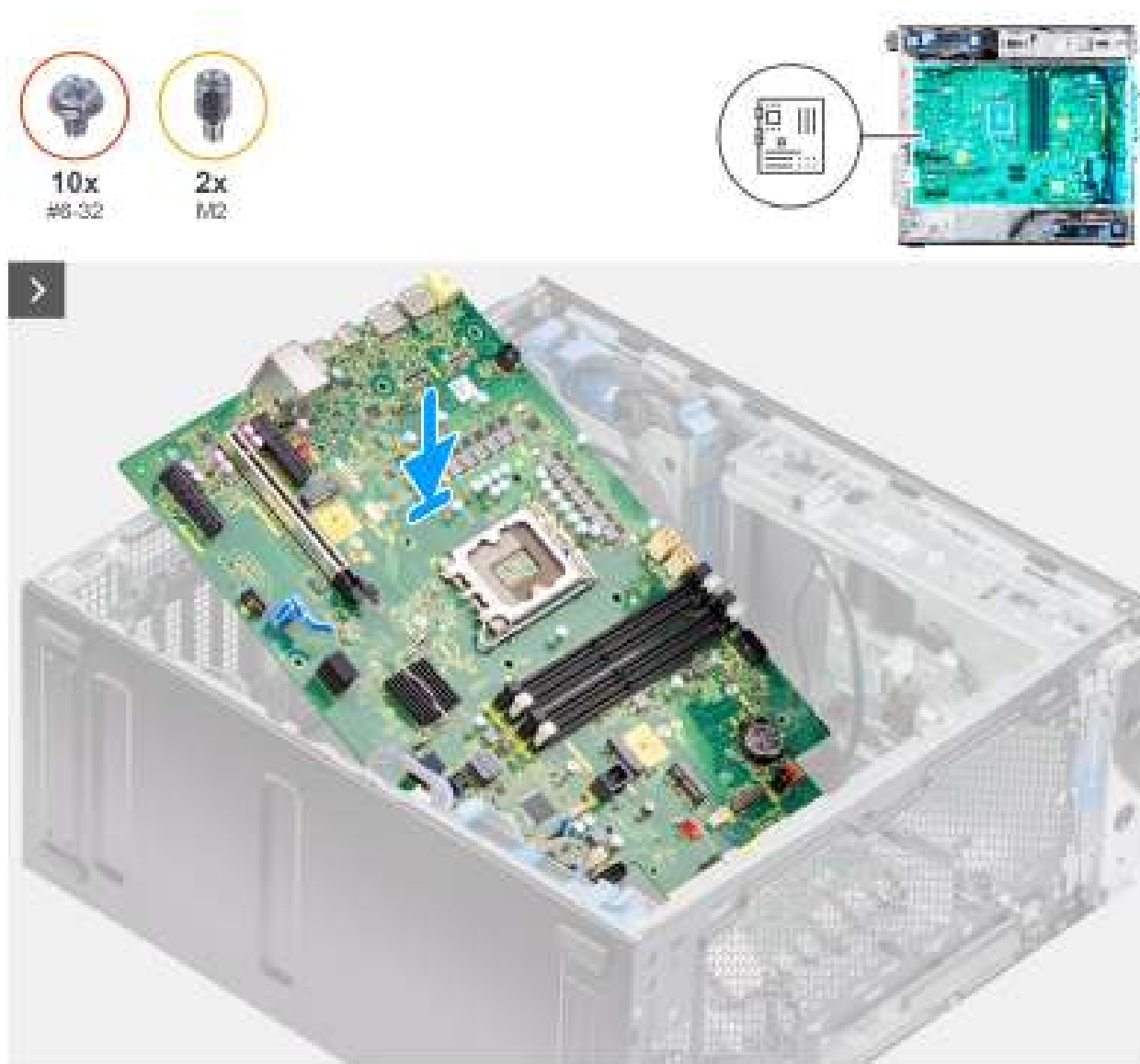
Figure 80. Installing the system board
