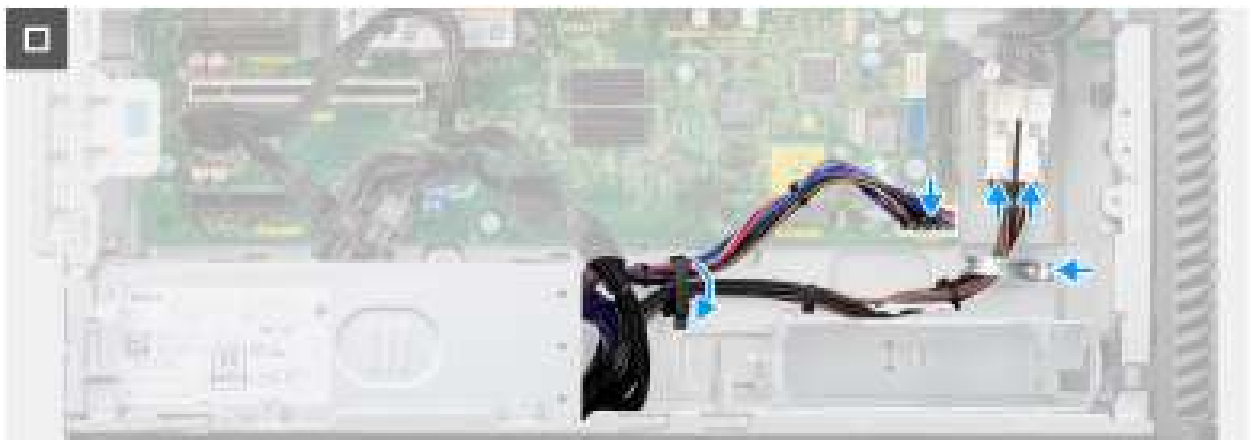
Figure 50. Installing the 1000W power-supply unit
