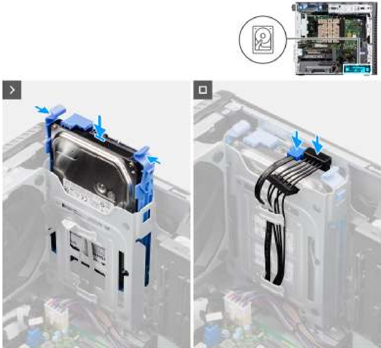
Figure 21. Installing the 3.5-inch hard drive assembly from Bay 1
