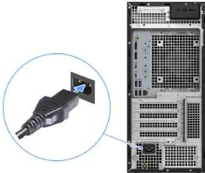
Figure 6. Connect the power cable
