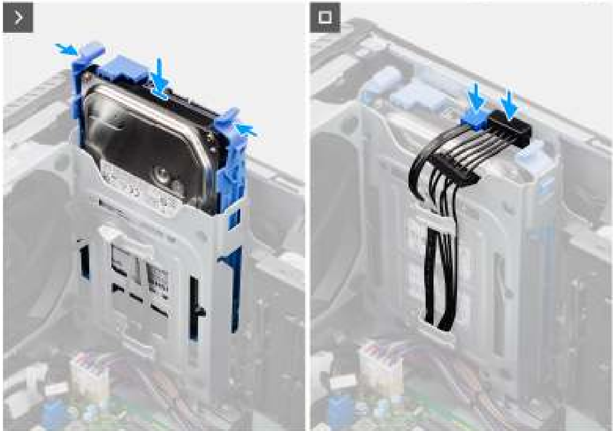
Figure 20. Installing the 3.5-inch hard drive assembly (Bay-2)
