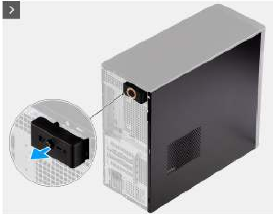
Figure 8. Removing the side cover
