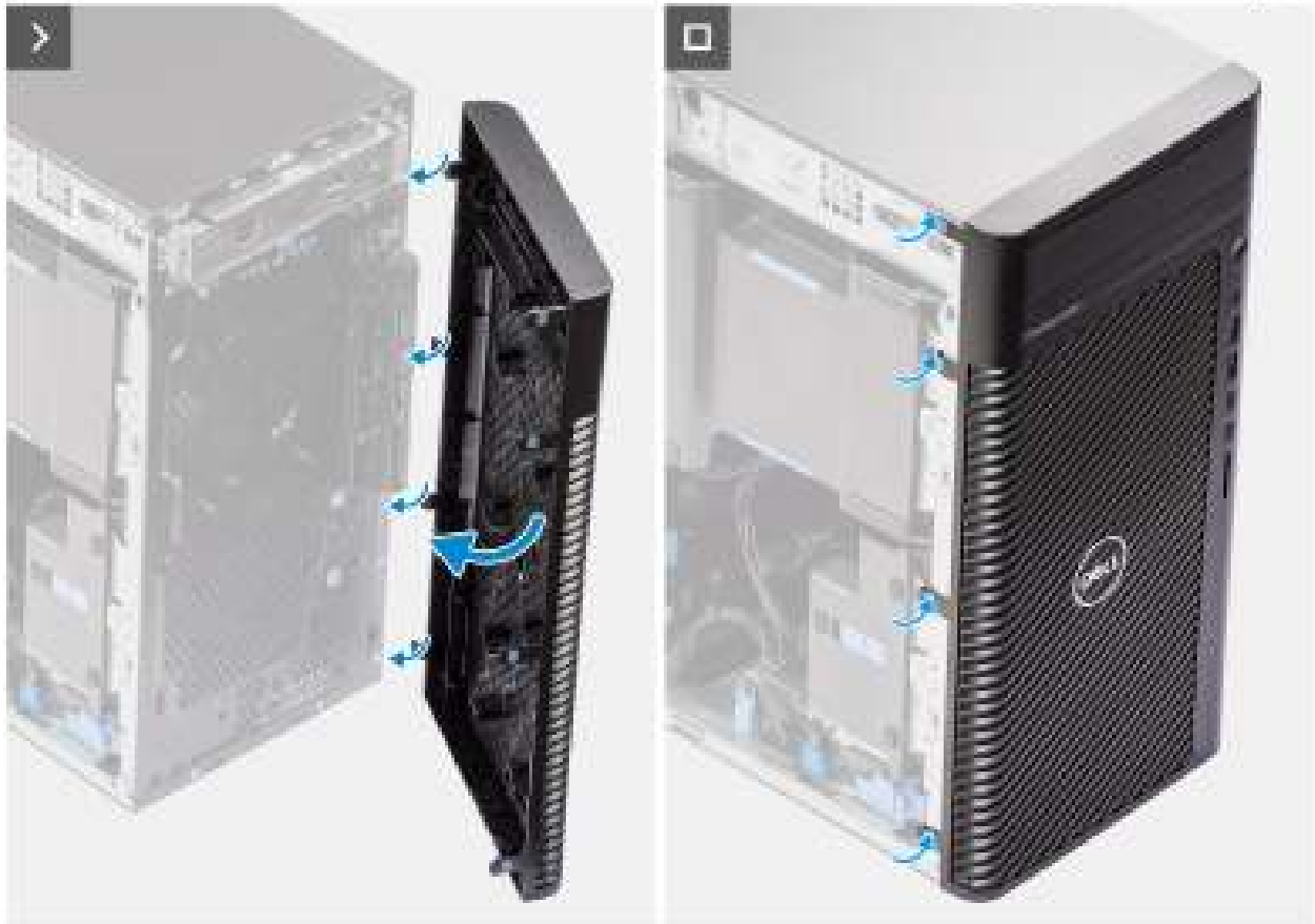
Figure 13. Installing the front bezel
