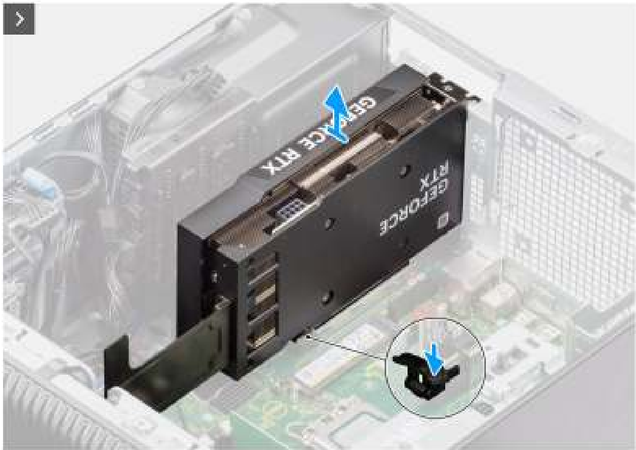
Figure 41. Removing the powered GPU
