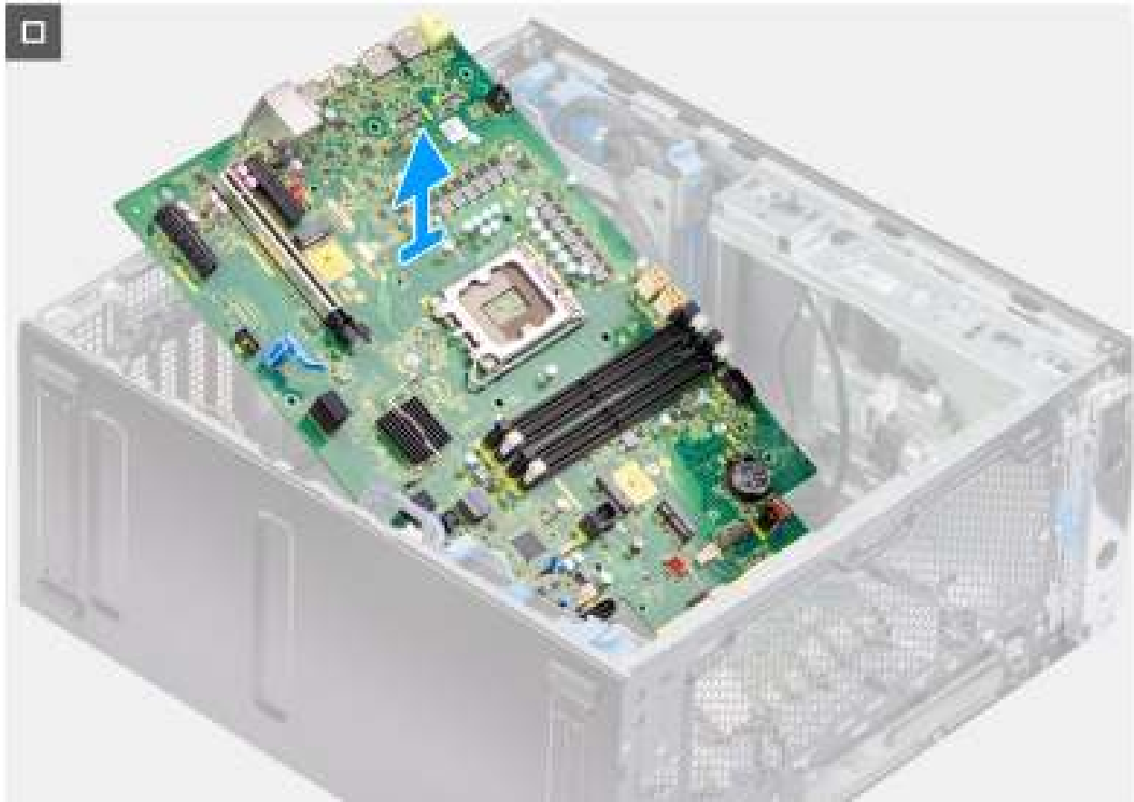
Figure 78. Removing the system board
