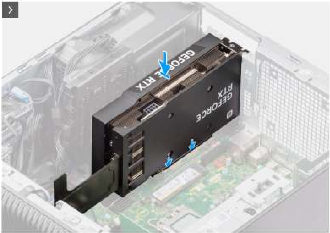
Figure 44. Installing the powered GPU
