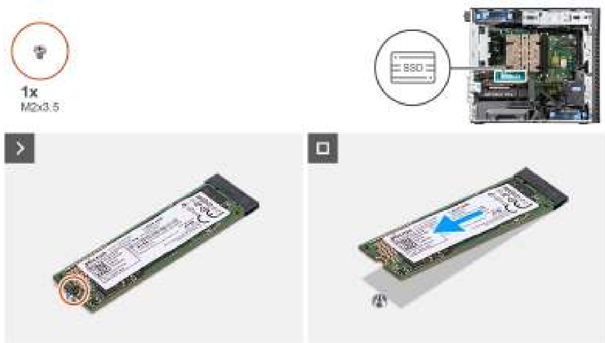
Figure 24. Removing the M.2 2280 PCIe solid state drive
