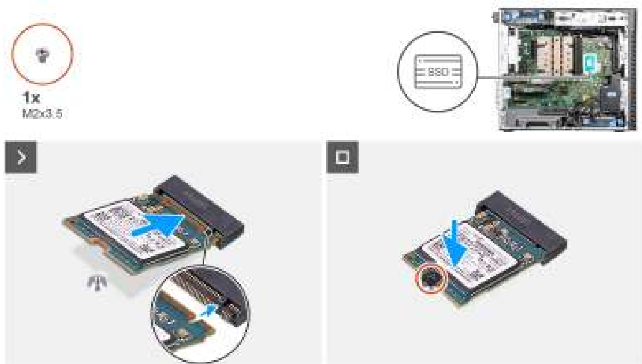
Figure 23. Installing the M.2 2230 PCIe solid state drive
