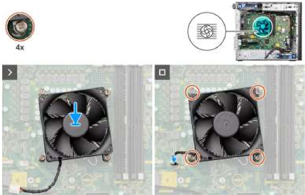
Figure 55. Installing the processor fan and 65 W heat-sink assembly
