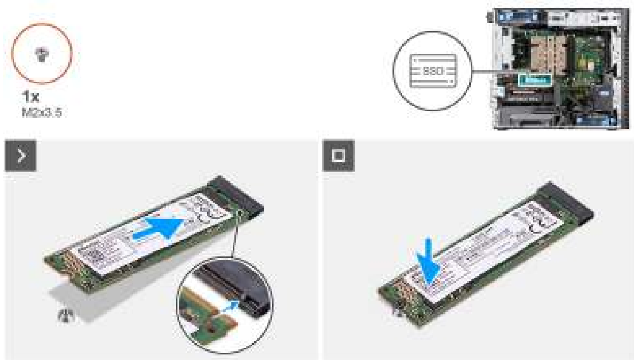
Figure 25. Installing the M.2 2280 PCIe solid state drive
