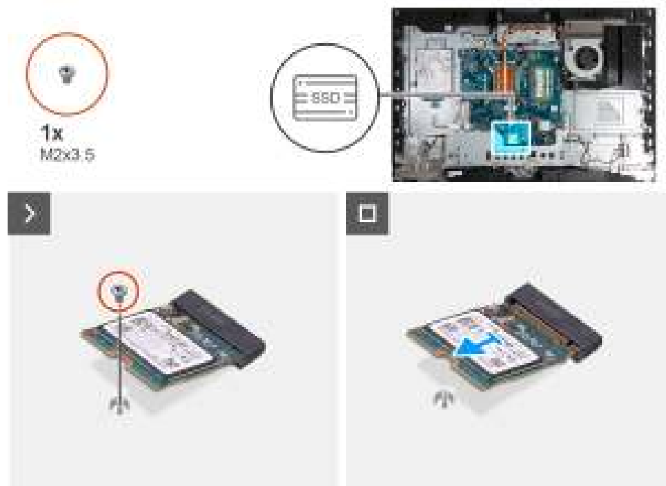
Figure 90. Removing the M.2 2230 solid-state drive
