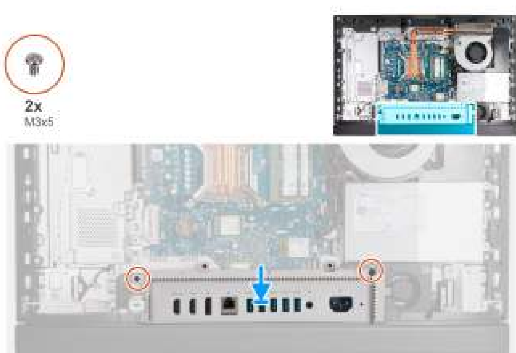
Figure 43. Installing the I/O cover
