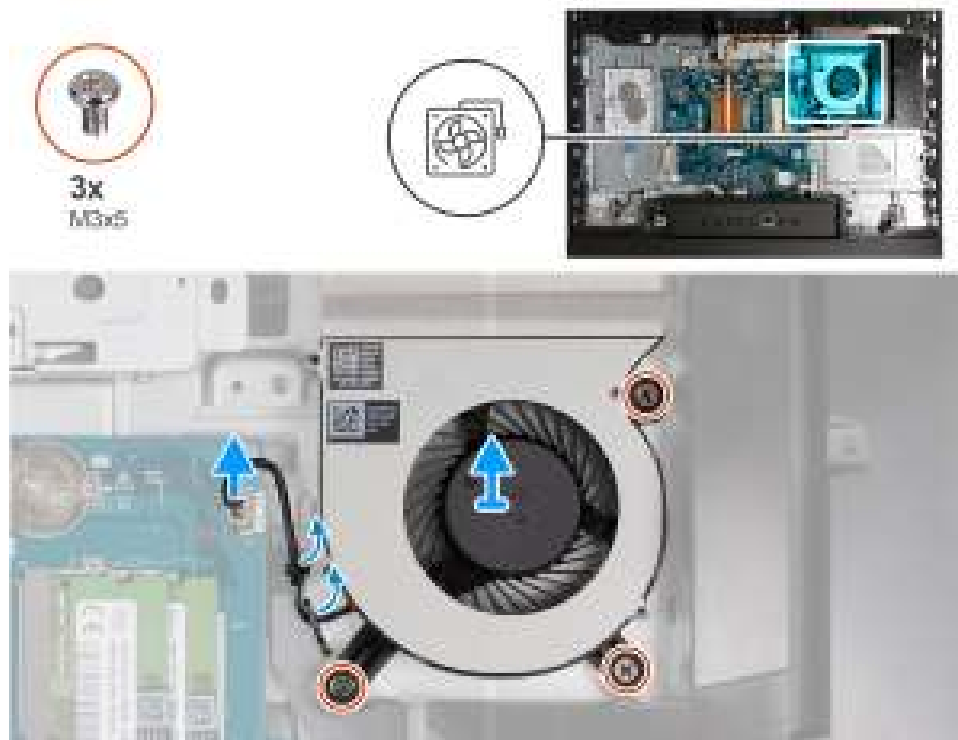
Figure 103. Removing the fan
