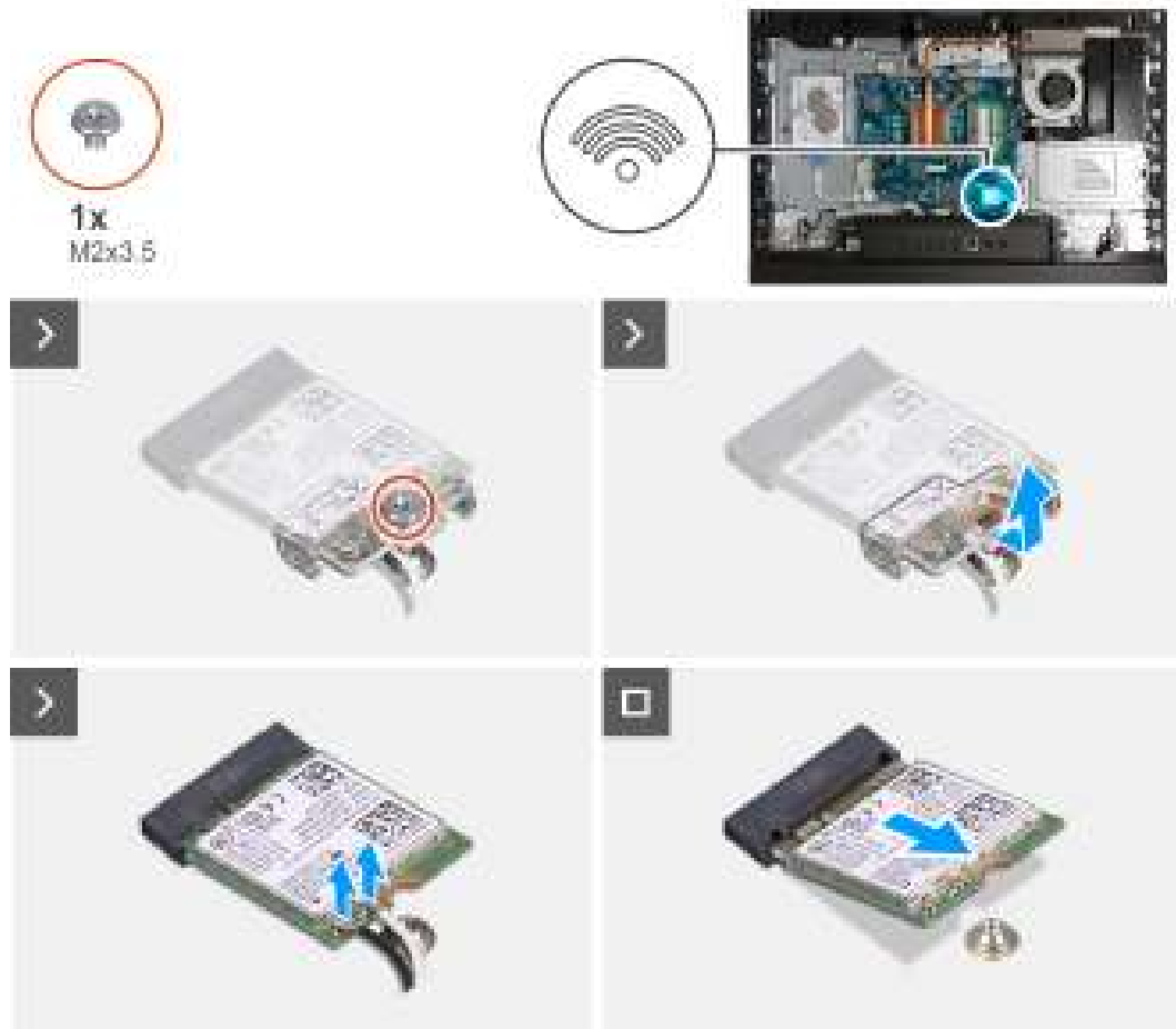
Figure 88. Removing the wireless card
