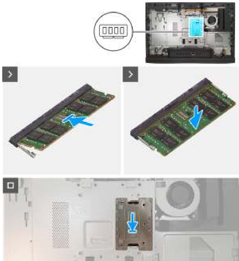
Figure 85. Installing the memory
