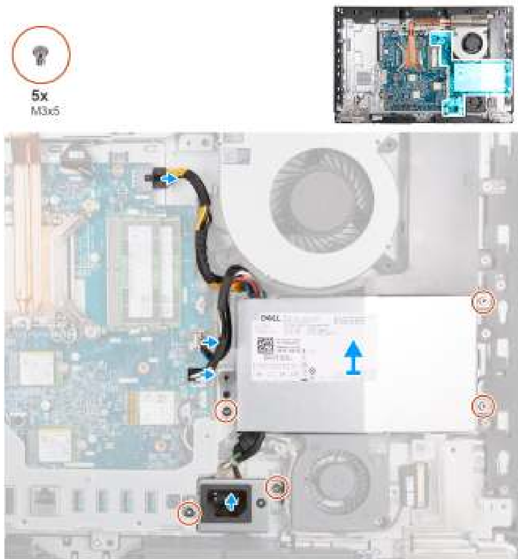
Figure 50. Removing the power-supply unit
