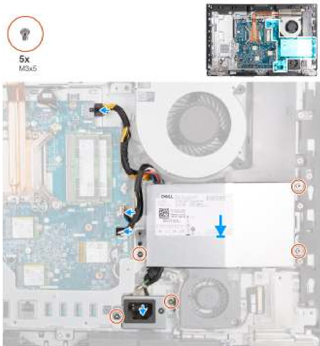
Figure 51. Installing the power-supply unit
