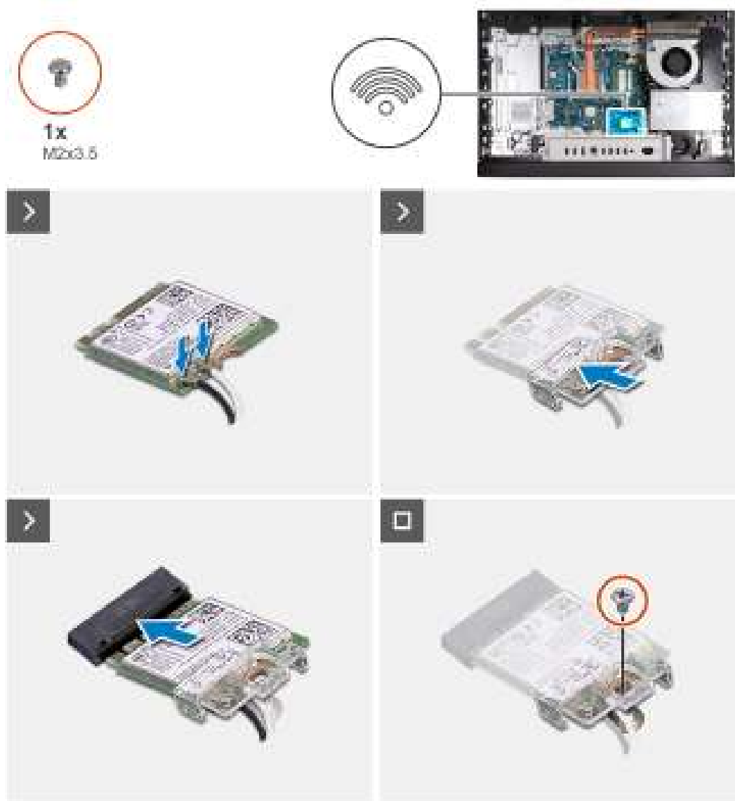
Figure 29. Installing the wireless card
