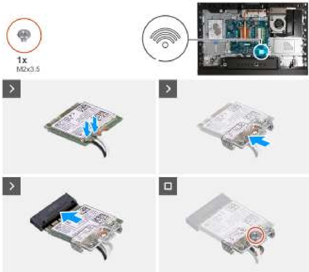
Figure 89. Installing the wireless card
