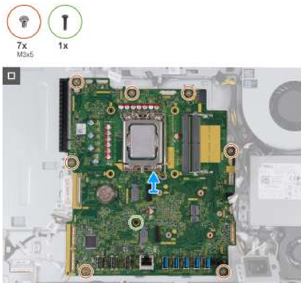
Figure 68. Removing the system board
