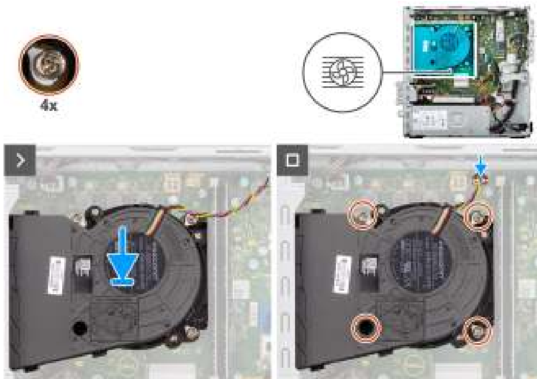
Figure 45. Installing the processor fan and heat-sink assembly
