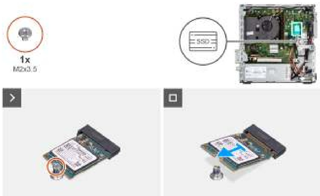
Figure 17. Removing the M.2 2230 solid-state drive
