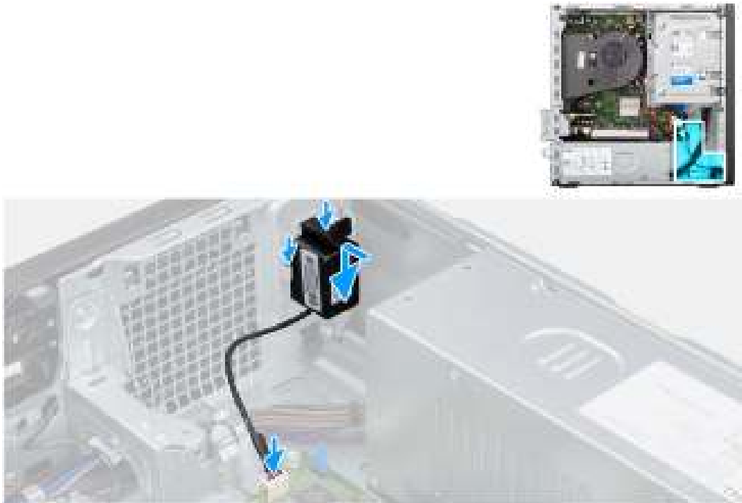
Figure 32. Installing the speaker
