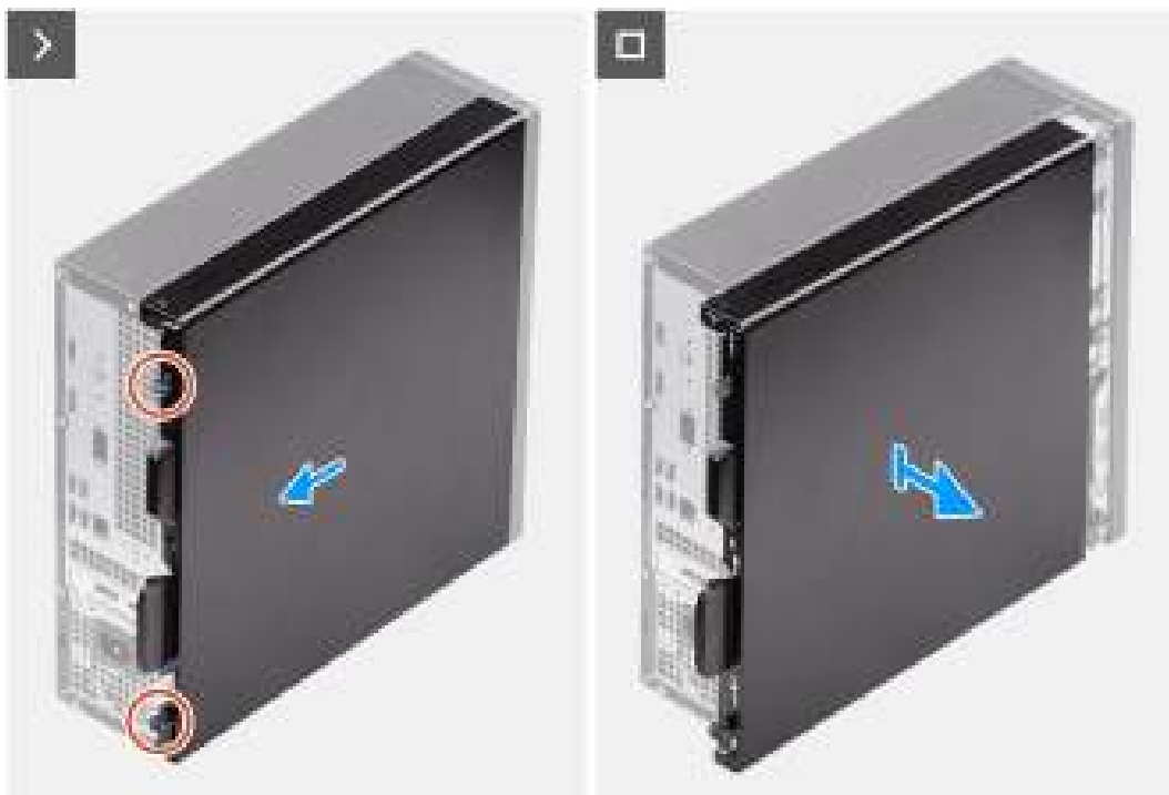
Figure 3. Removing the side cover
