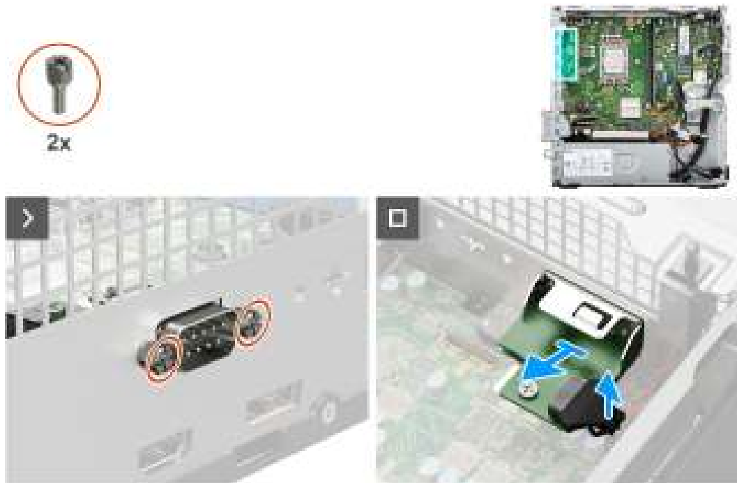
Figure 48. Removing the serial module
