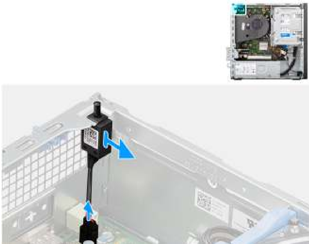
Figure 33. Removing the intrusion switch
