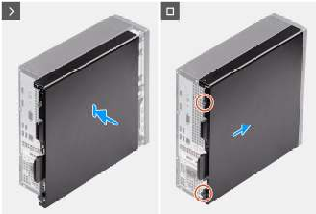
Figure 4. Installing the side cover
