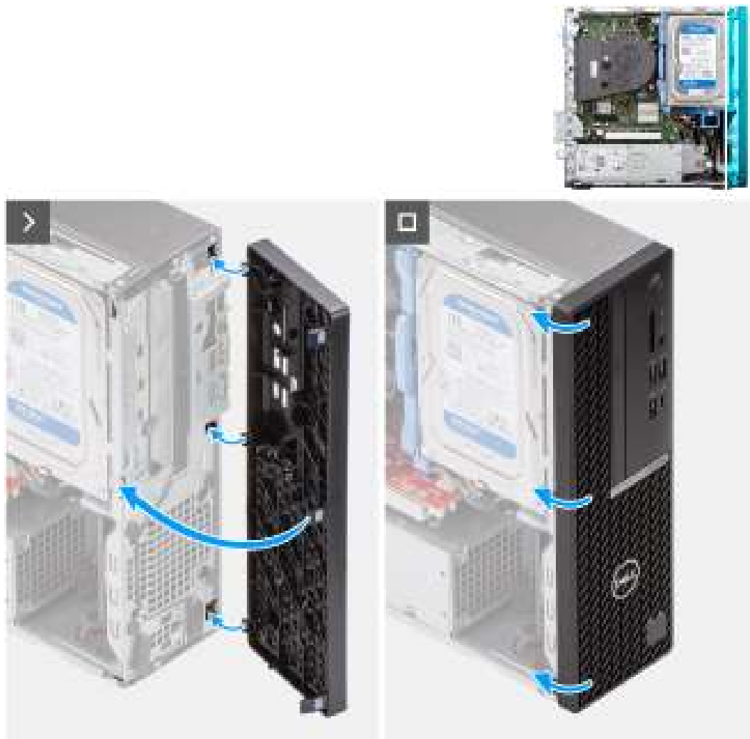
Figure 8. Installing the front bezel
