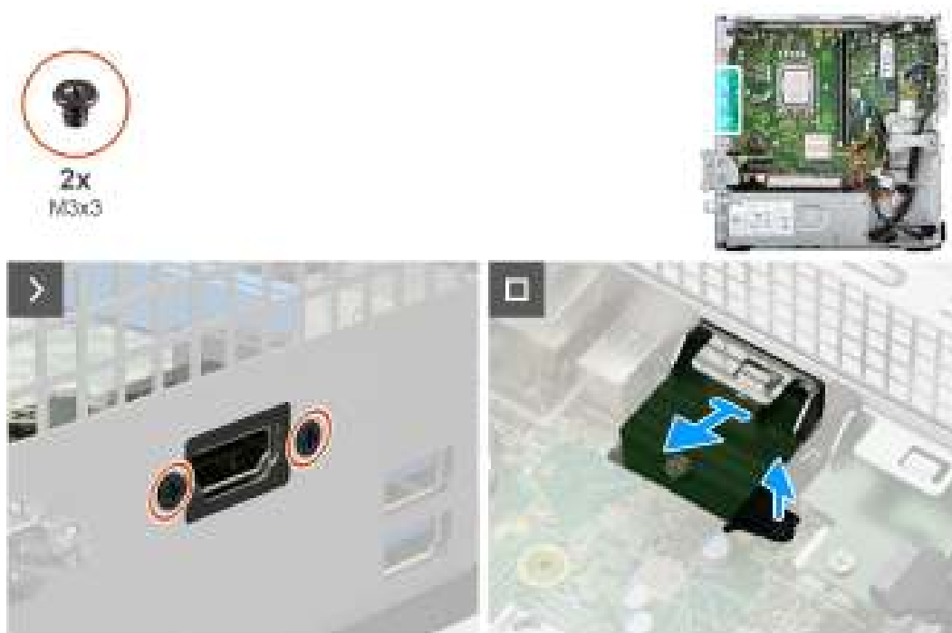
Figure 54. Removing the HDMI module
