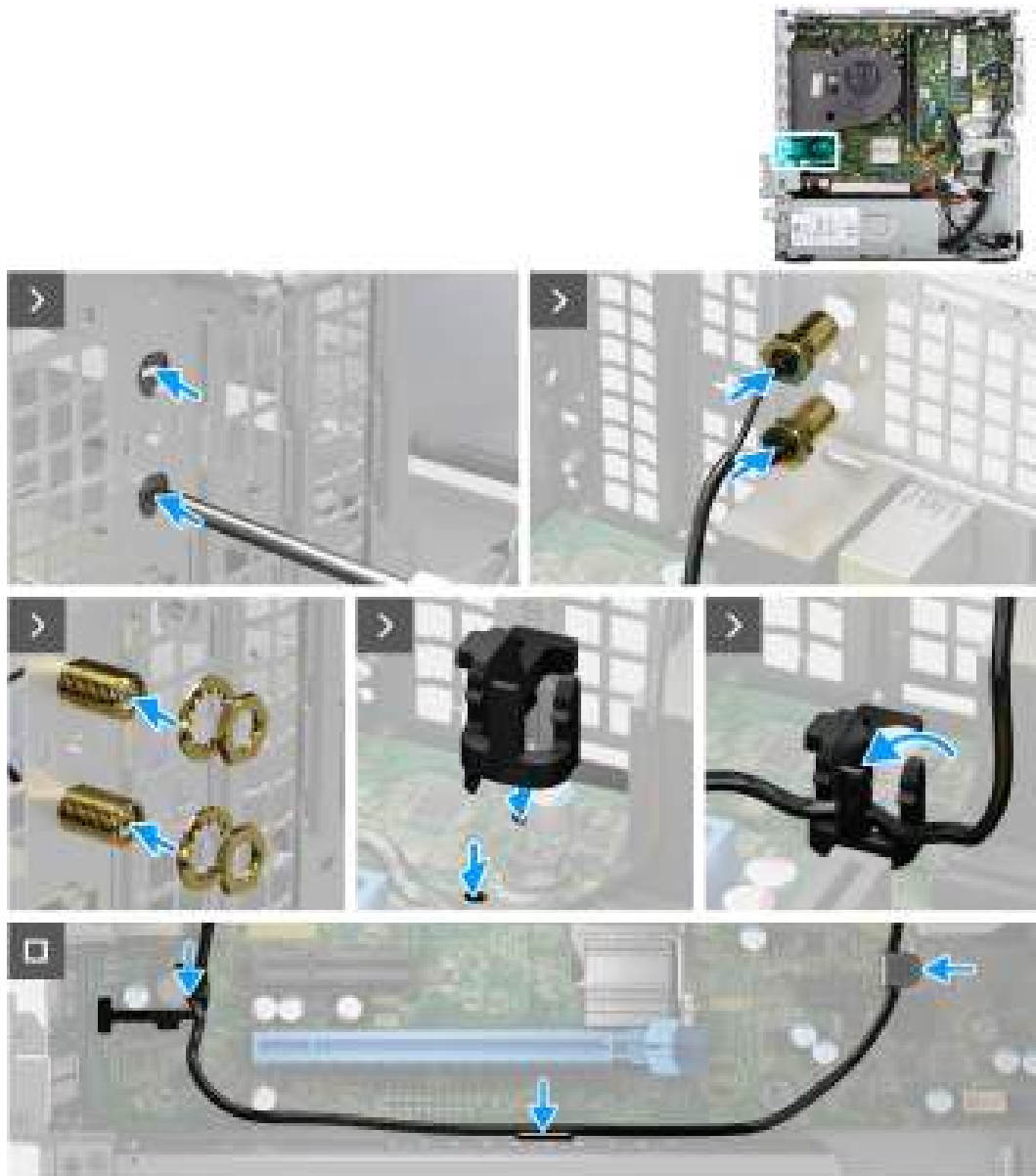
Figure 41. Installing the external SMA antenna module
