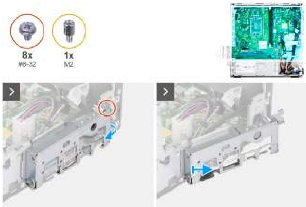
Figure 57. Removing the system board
