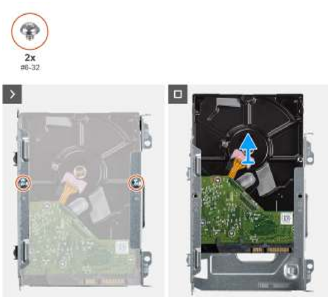
Figure 9. Removing the 3.5-inch hard drive
