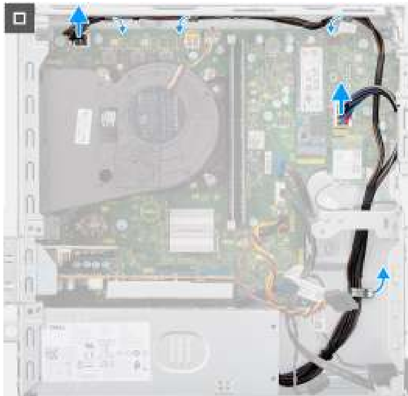
Figure 43. Installing the power-supply unit
