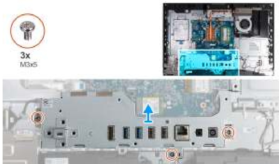
Figure 105. Removing the I/O bracket
