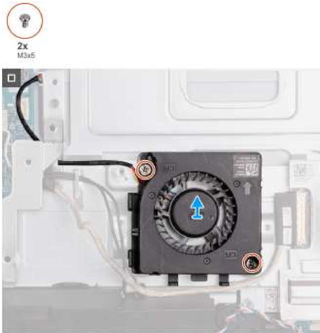
Figure 54. Removing the power-supply fan
