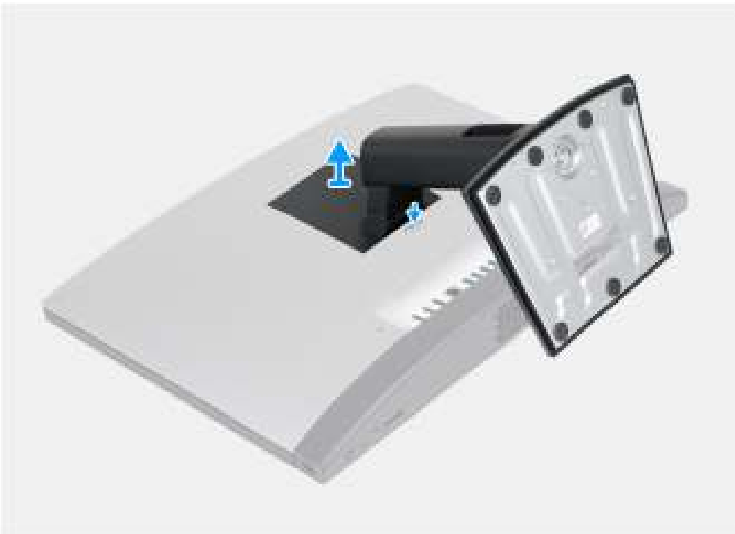
Figure 19. Removing the Fixed Stand
