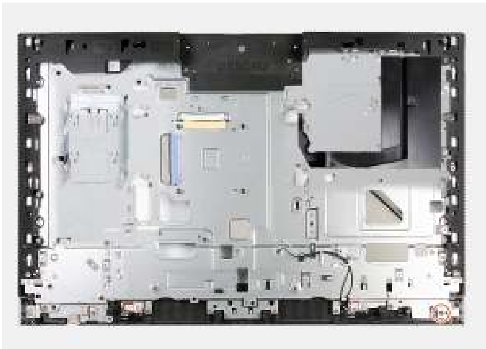
Figure 124. Installing the display-assembly base
