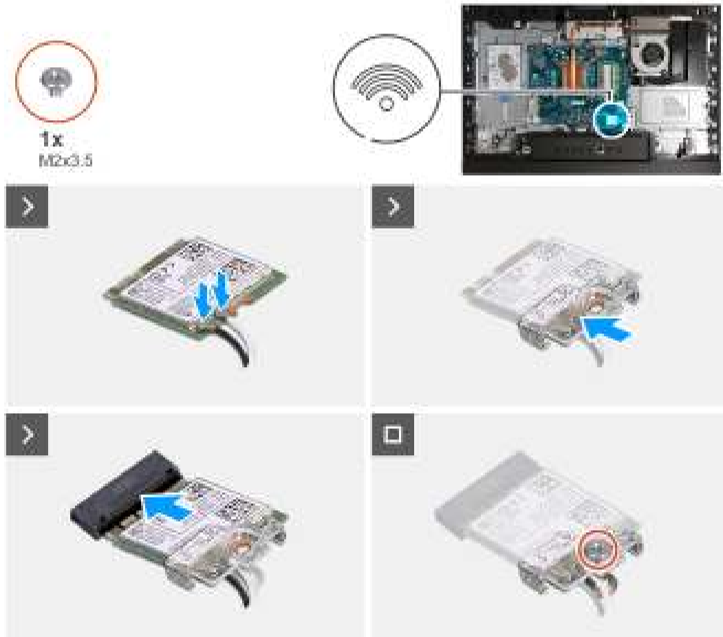
Figure 89. Installing the wireless card
