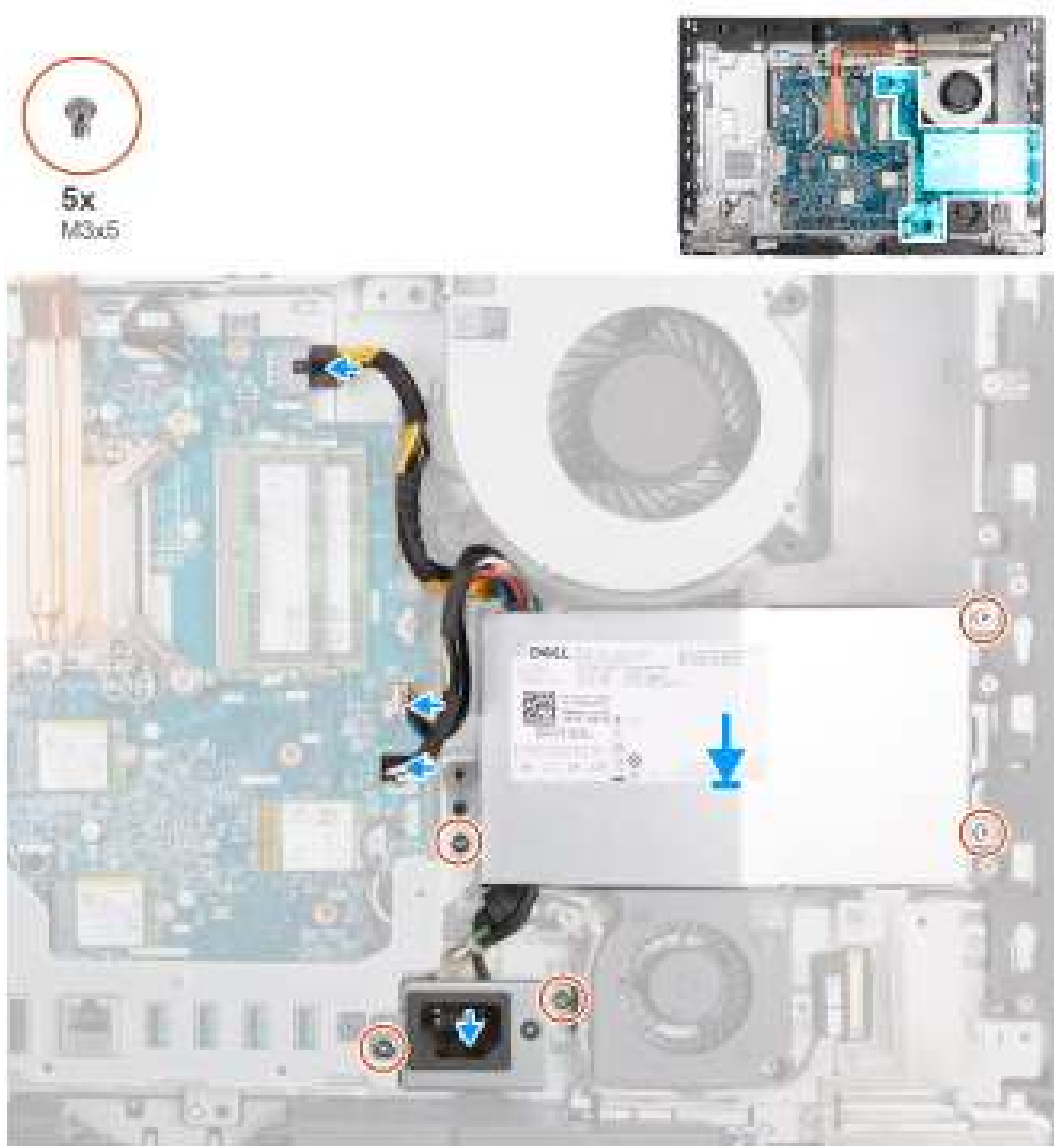
Figure 51. Installing the power-supply unit
