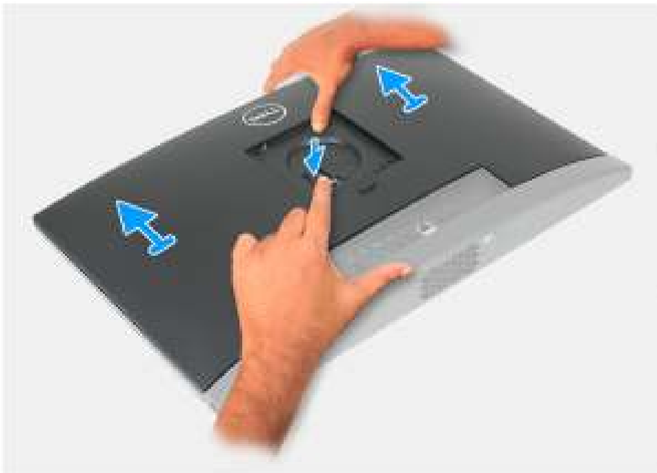
Figure 82. Removing the back cover
