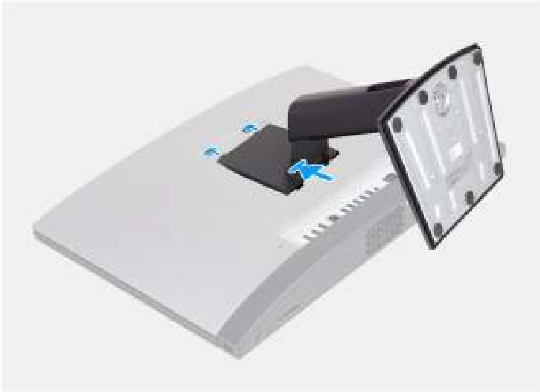
Figure 21. Installing the Fixed Stand
