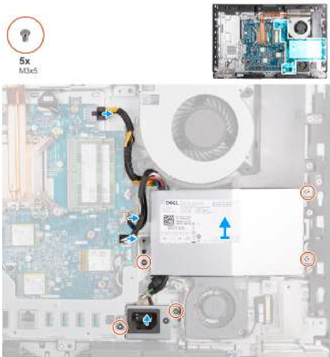
Figure 50. Removing the power-supply unit
