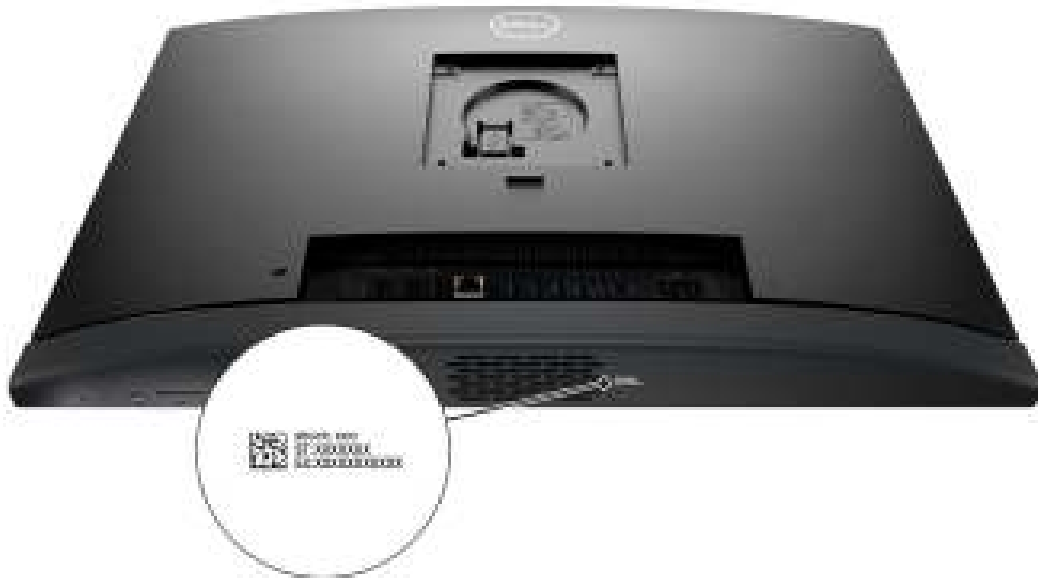
Figure 9. Service tag location of your OptiPlex All-in-One 7420
