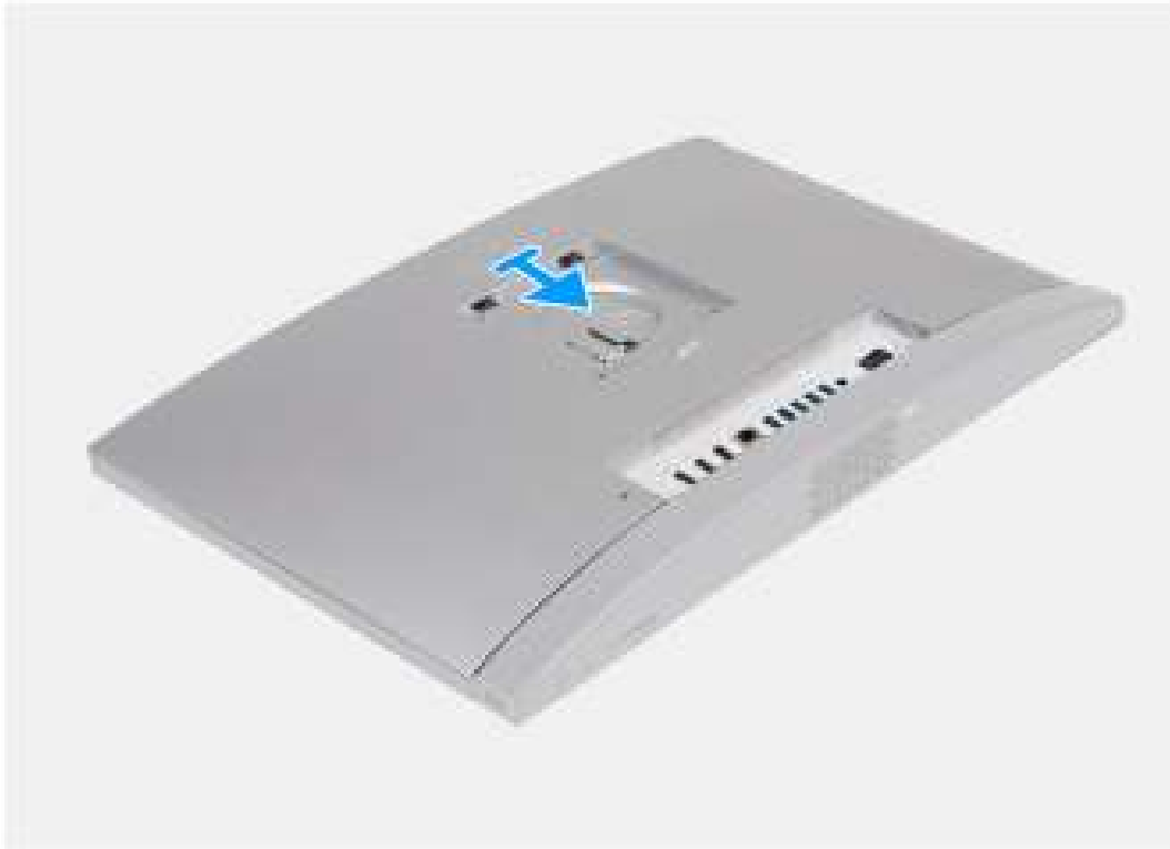
Figure 23. Installing the back cover
