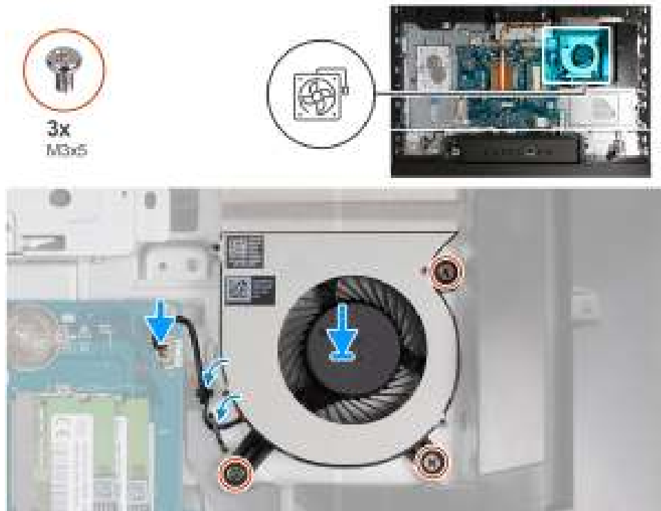
Figure 104. Installing the fan
