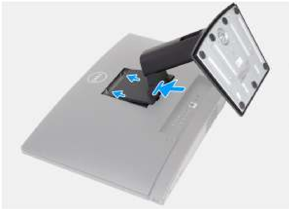
Figure 80. Installing the stand
