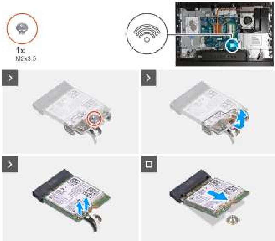
Figure 88. Removing the wireless card
