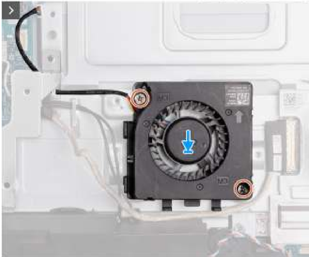
Figure 55. Installing the power-supply fan
