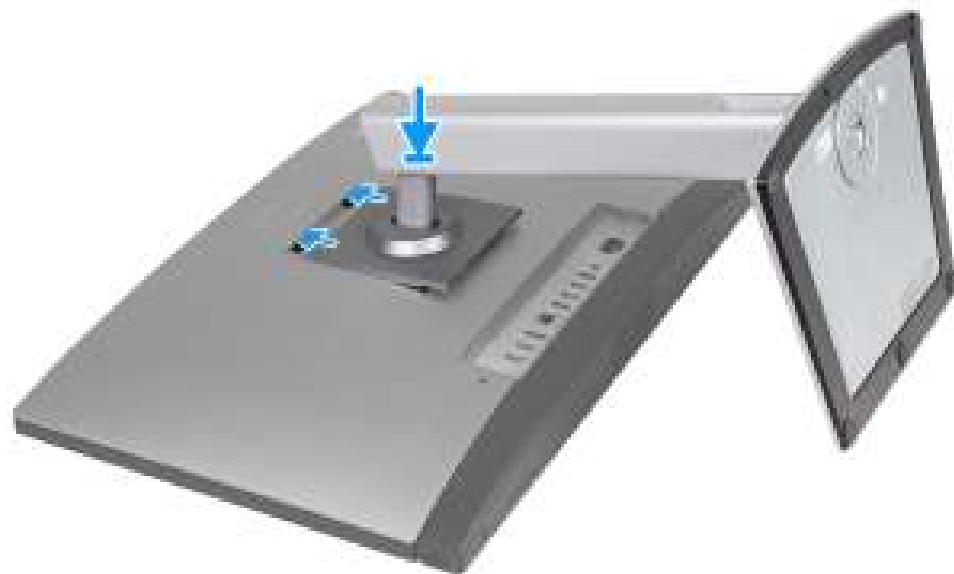
Figure 81. Installing the stand
