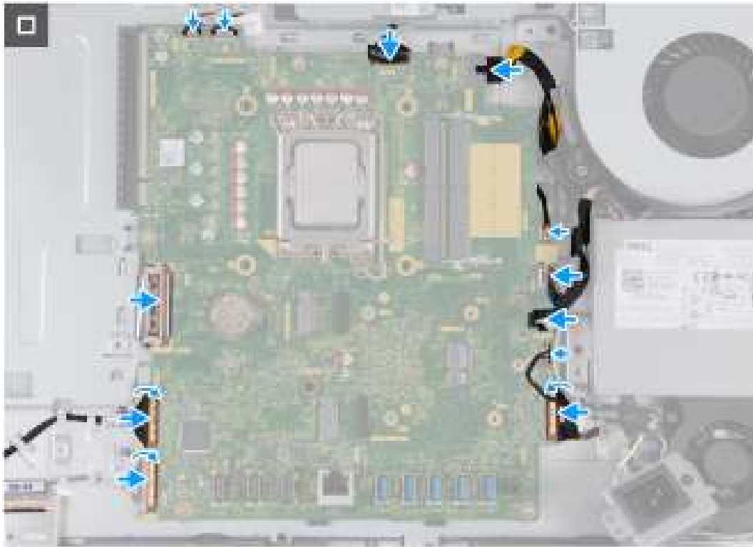
Figure 71. Installing the system board
