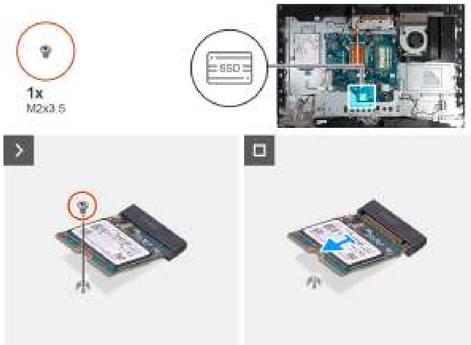
Figure 90. Removing the M.2 2230 solid-state drive
