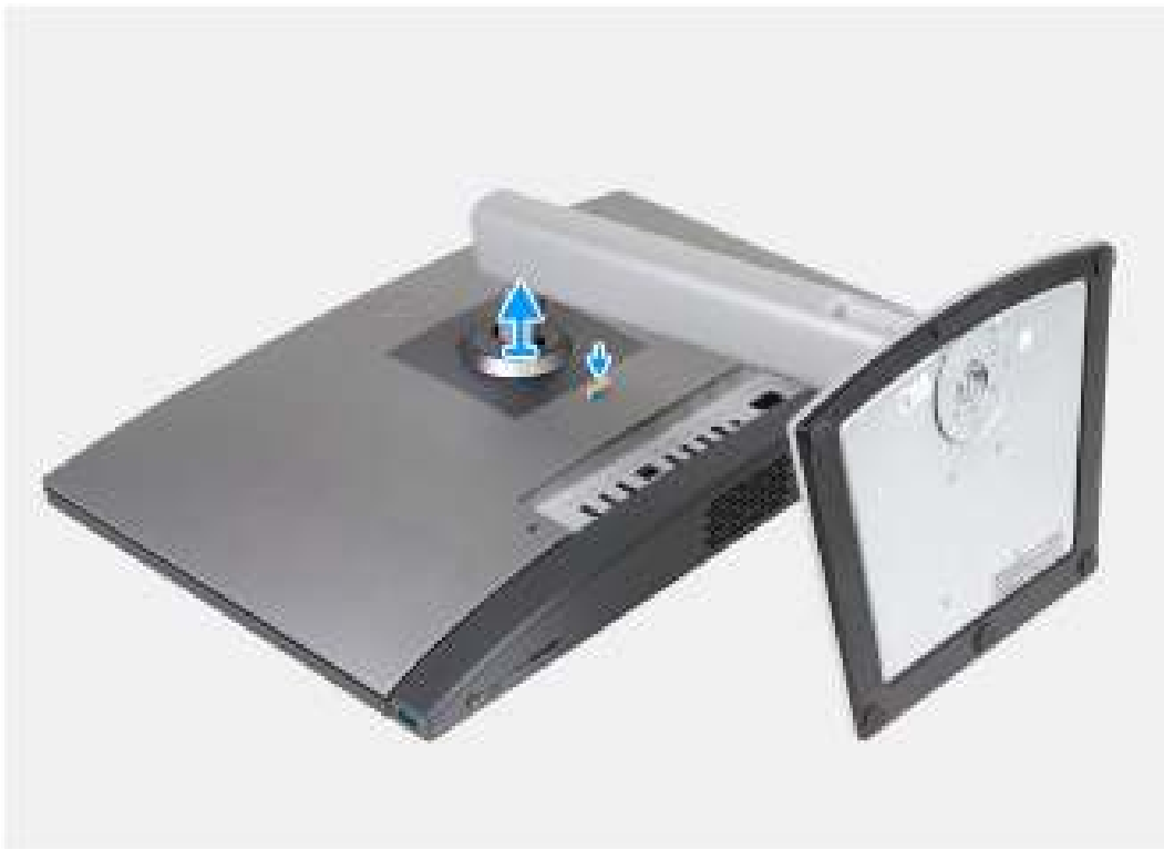
Figure 79. Removing the stand
