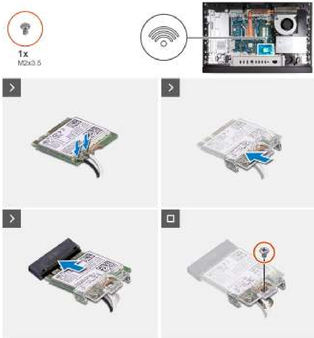
Figure 29. Installing the wireless card
