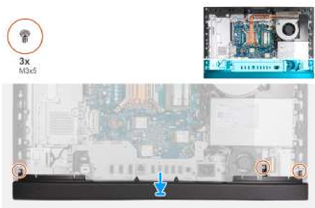
Figure 45. Installing the bottom cover
