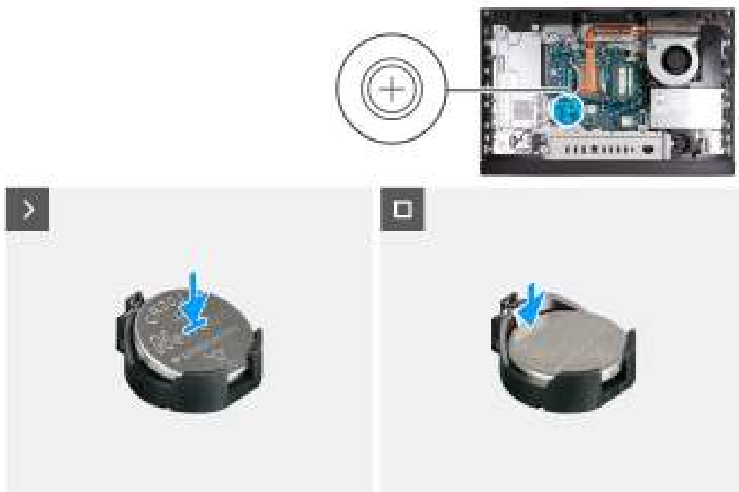
Figure 41. Installing the coin-cell battery
