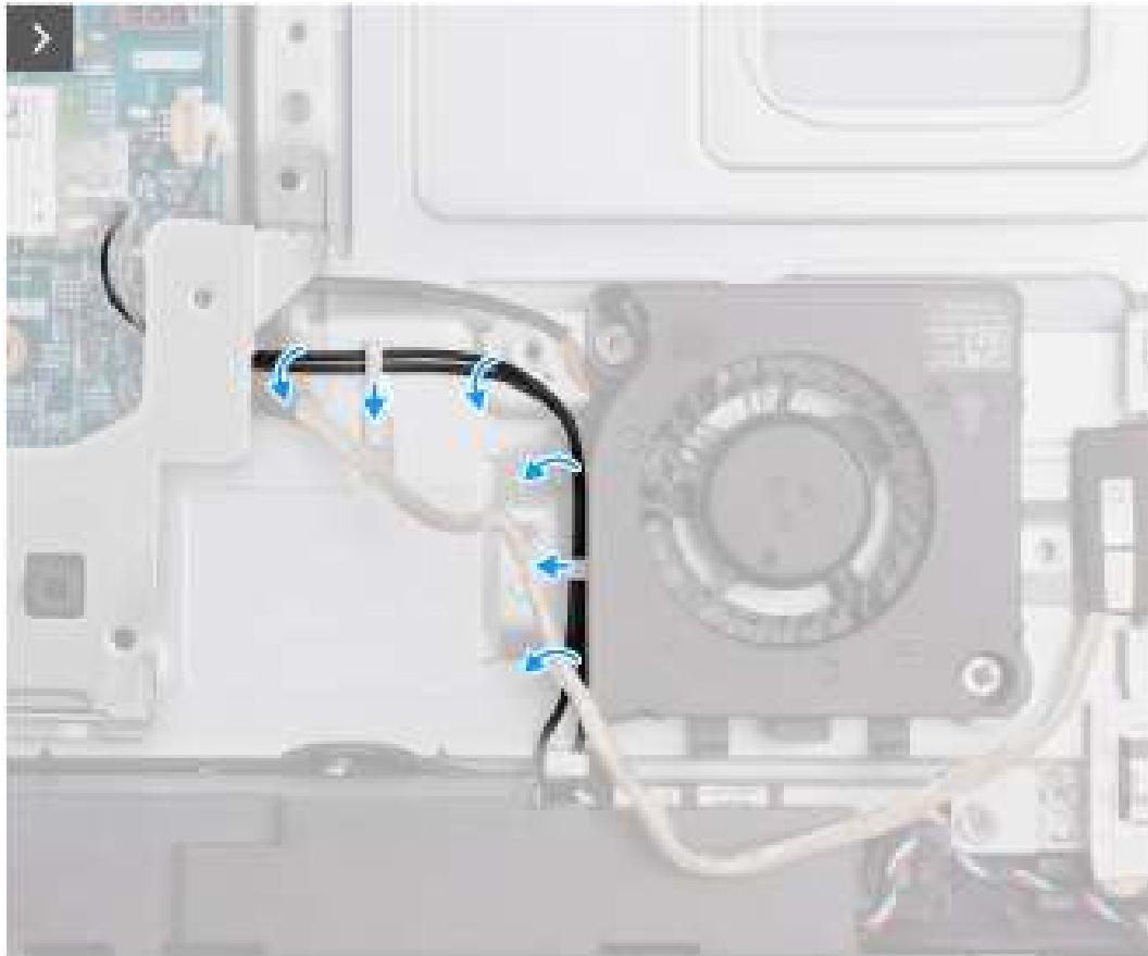
Figure 53. Removing the power-supply fan
