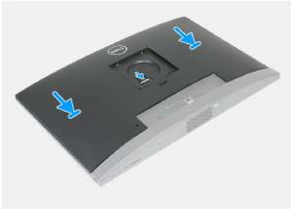
Figure 83. Installing the back cover
