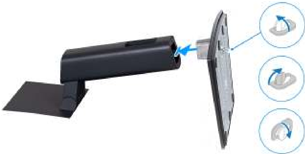
Figure 10. Installing the stand base
