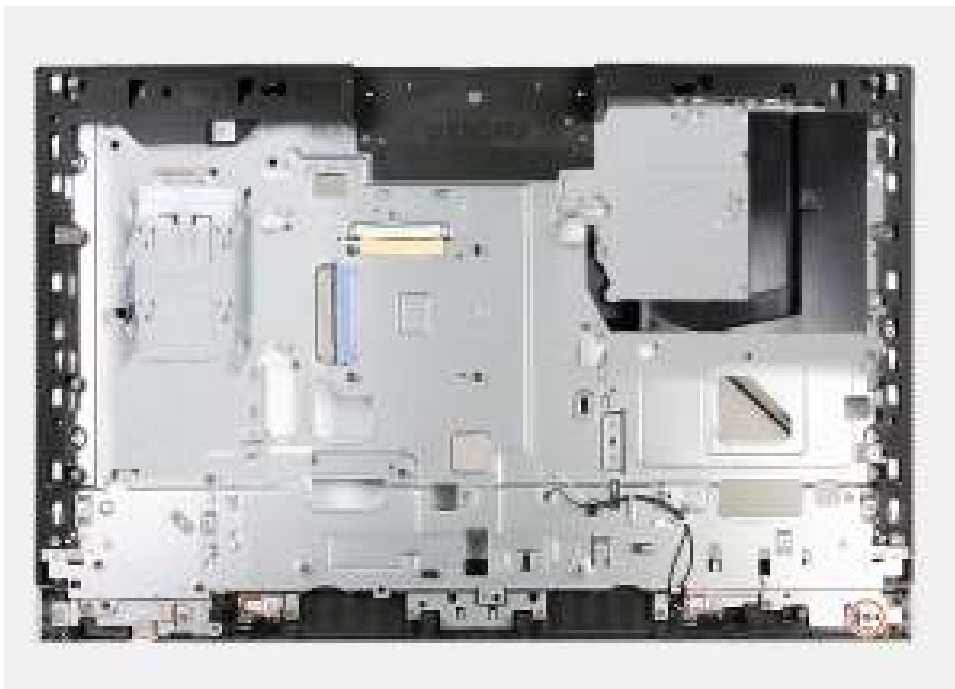
Figure 123. Removing the display-assembly base
