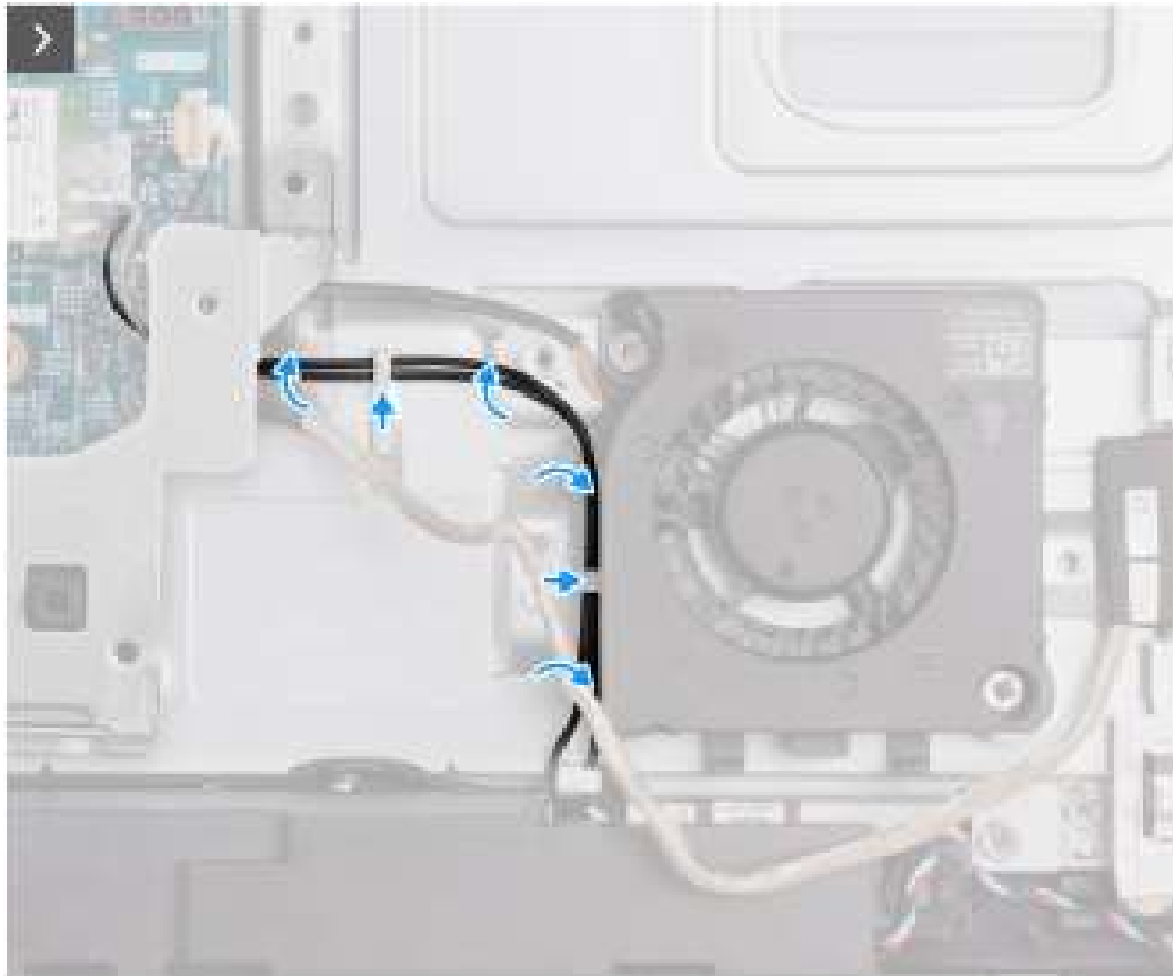
Figure 56. Installing the power-supply fan
