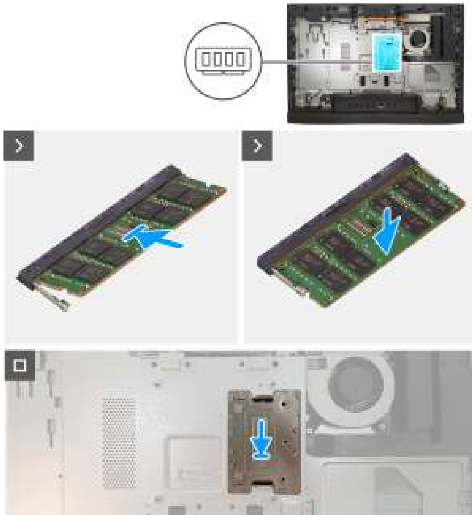
Figure 85. Installing the memory
