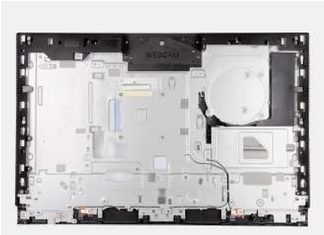
Figure 76. Removing the display-assembly base
