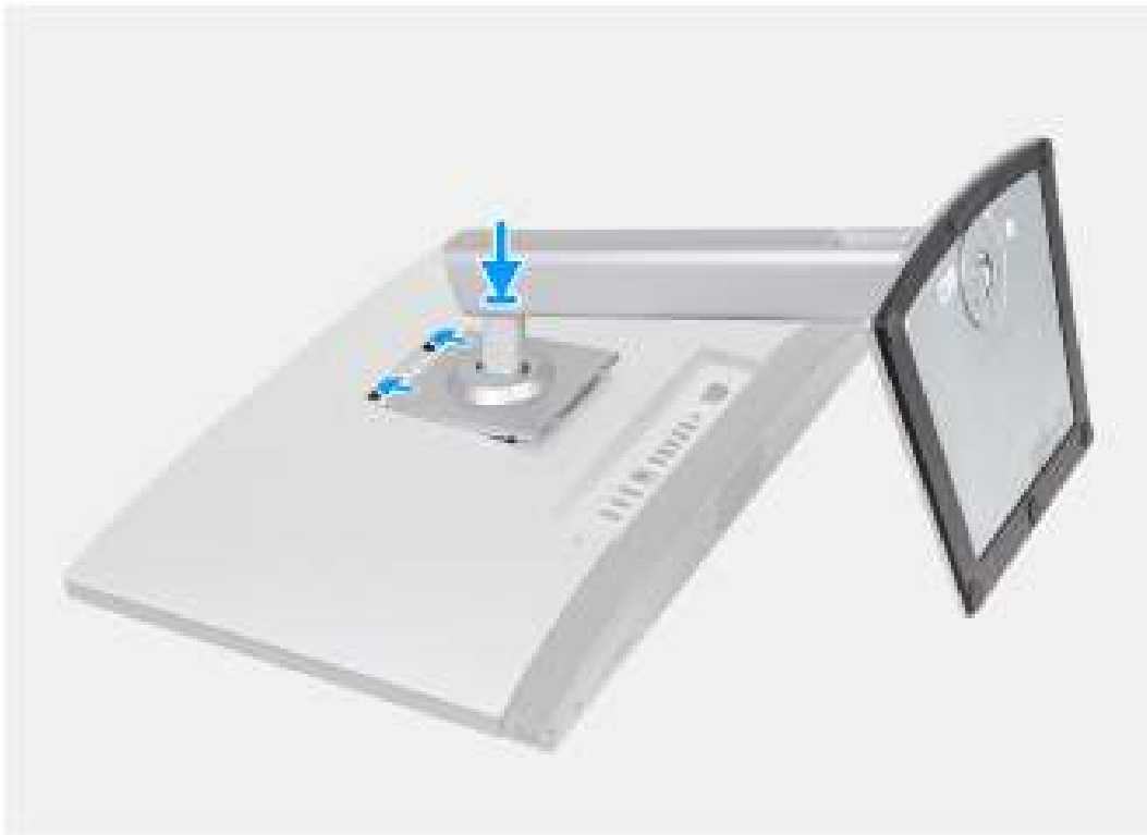
Figure 20. Installing the Height Adjustable Stand (HAS)
