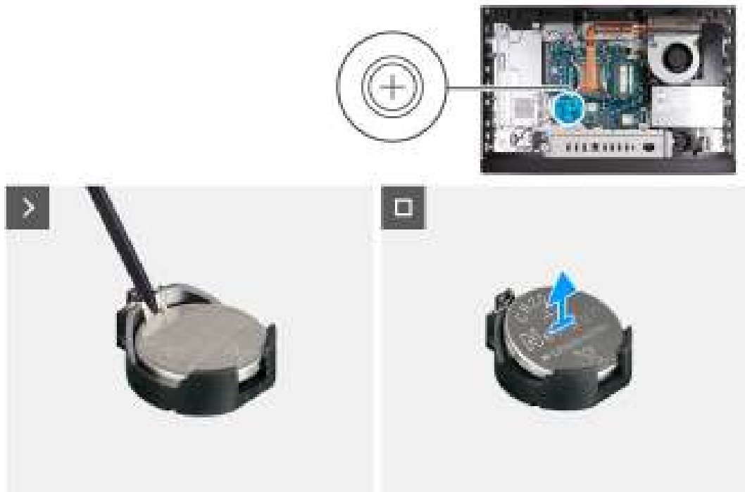
Figure 40. Removing the coin-cell battery
