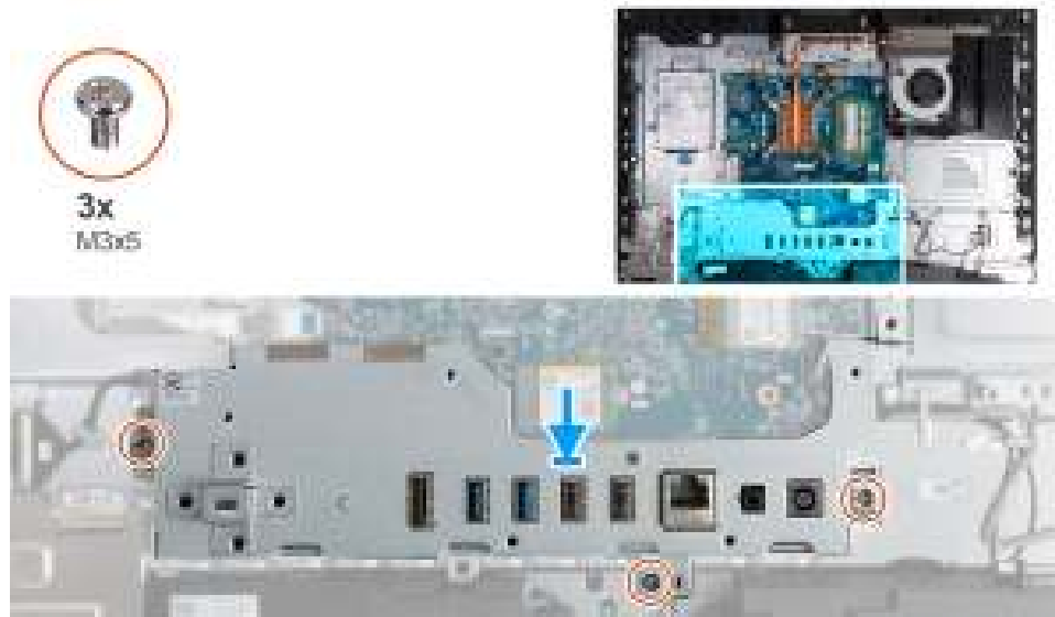
Figure 106. Installing the I/O bracket
