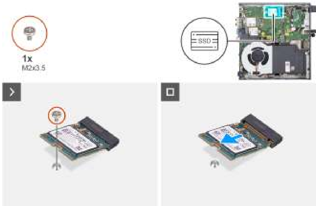
Figure 21. Removing the M.2 2230 solid-state drive from slot 1
