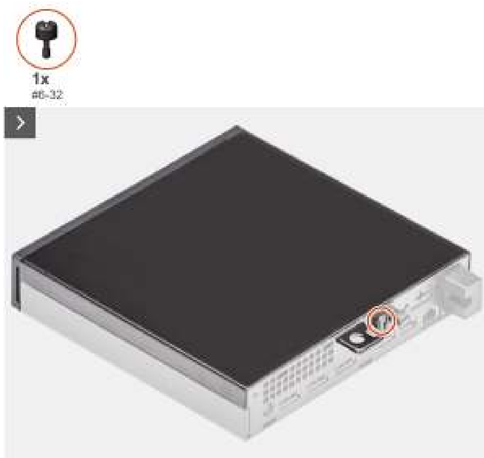
Figure 9. Removing the side cover
