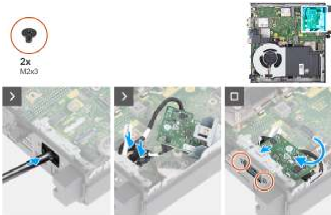
Figure 39. Installing the optional Type-C module
