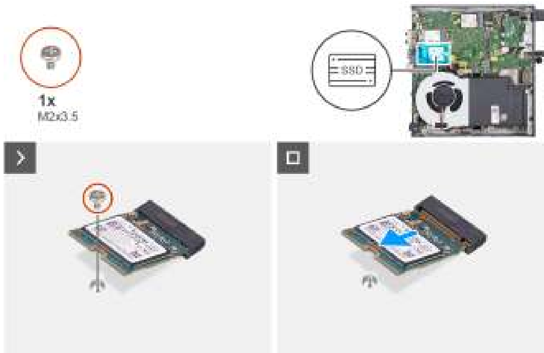
Figure 19. Removing the 2230 solid-state drive from slot 0
