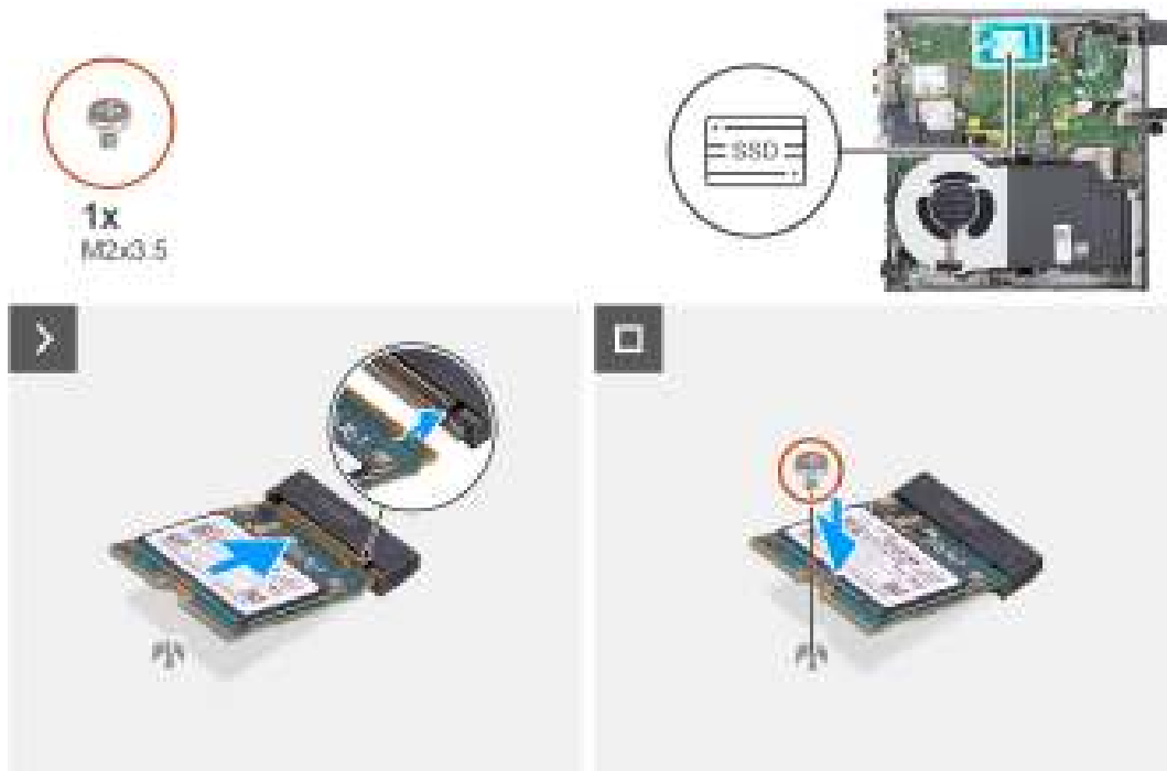
Figure 22. Installing the M.2 2230 solid-state drive in slot 1
