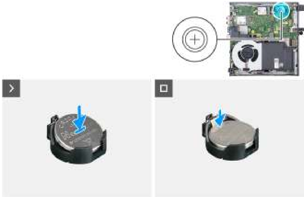
Figure 14. Installing the coin-cell battery
