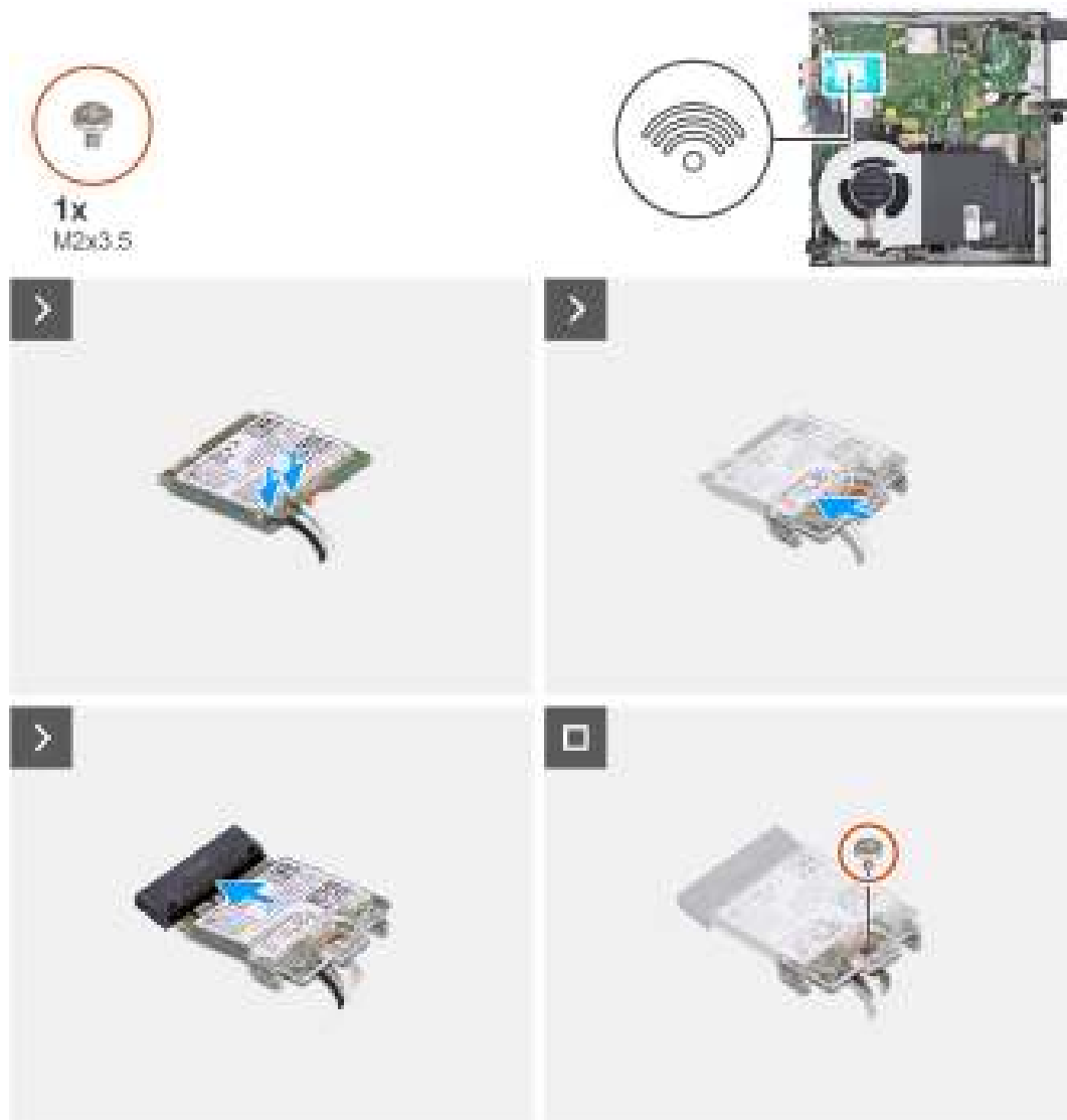
Figure 29. Installing the wireless card
