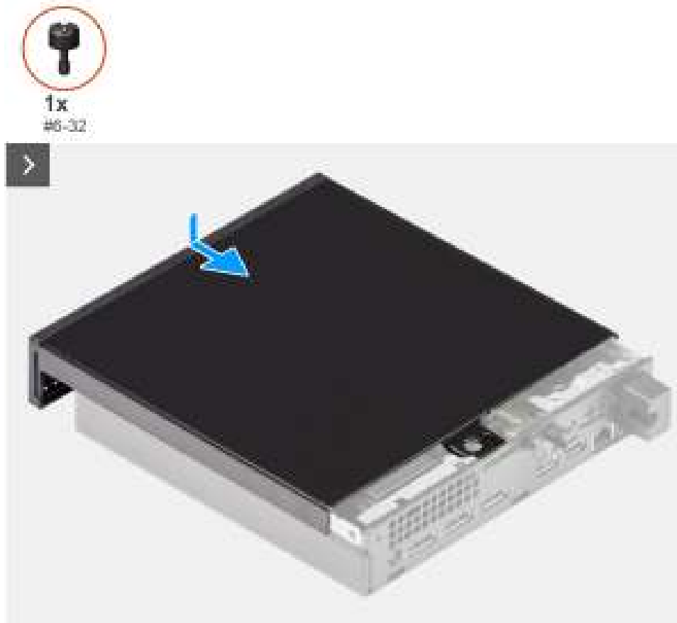
Figure 11. Installing the side cover
