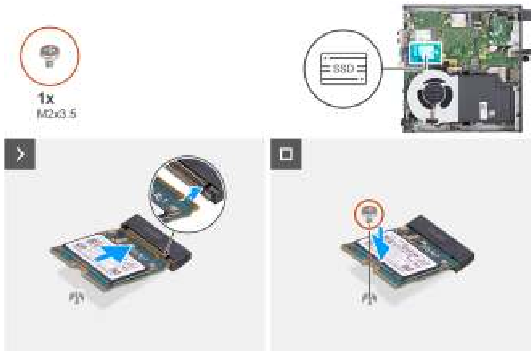
Figure 20. Installing the 2230 solid-state drive in slot 0
