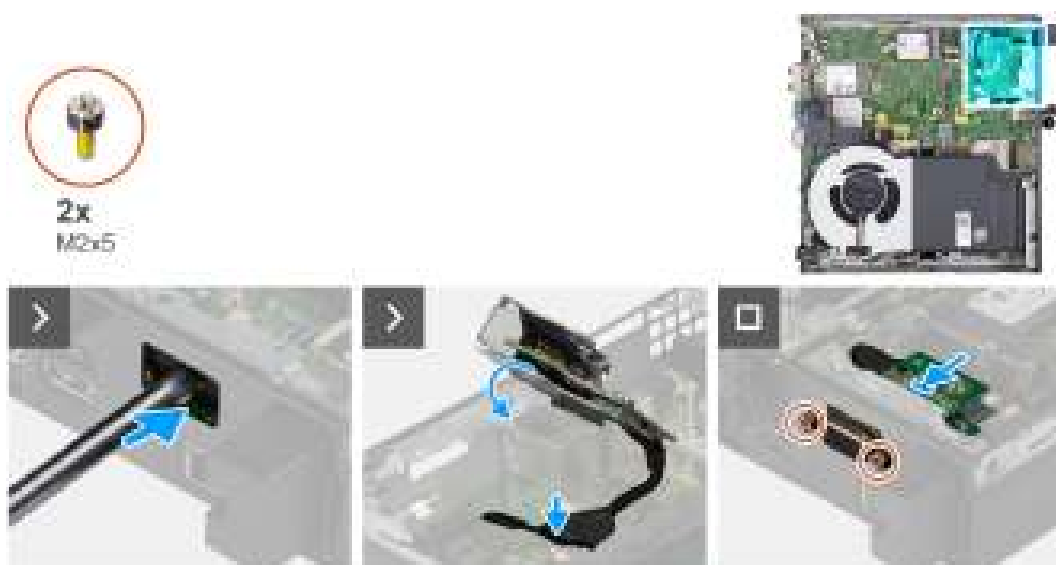
Figure 37. Installing optional I/O module (VGA or Serial)
