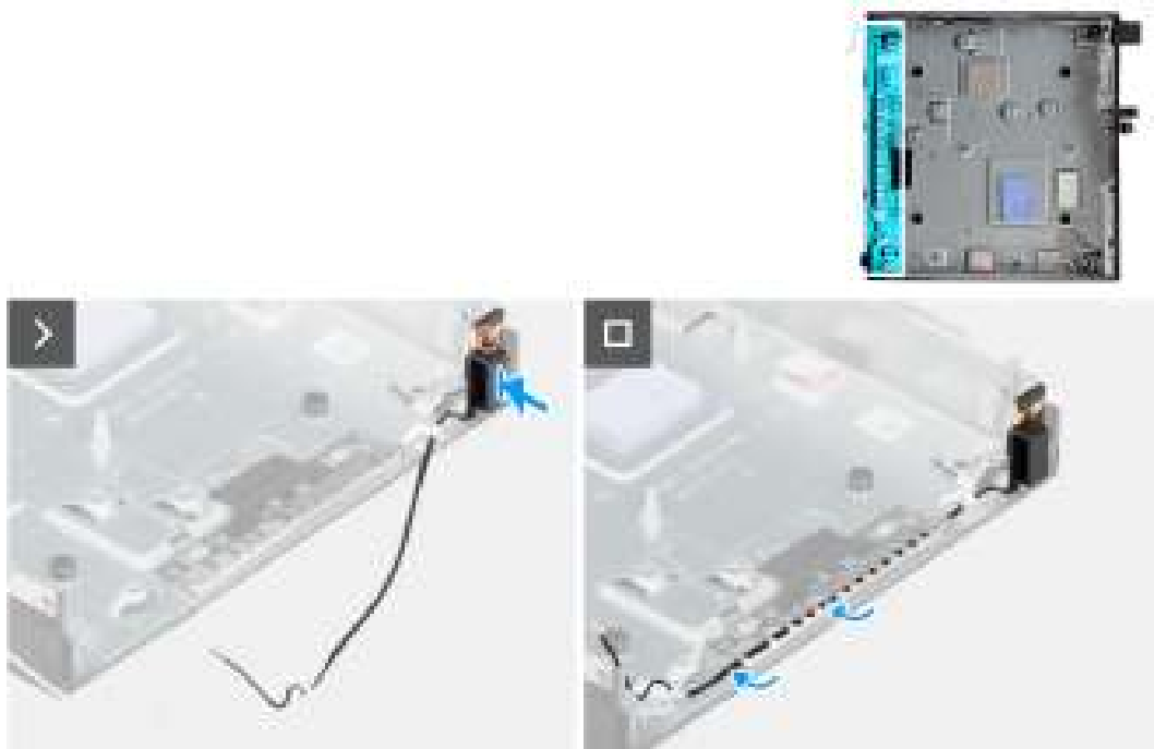
Figure 53. Installing the antenna module (black cable)
