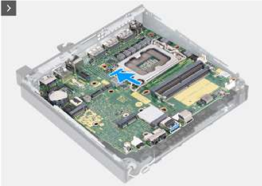
Figure 48. Installing the system board
