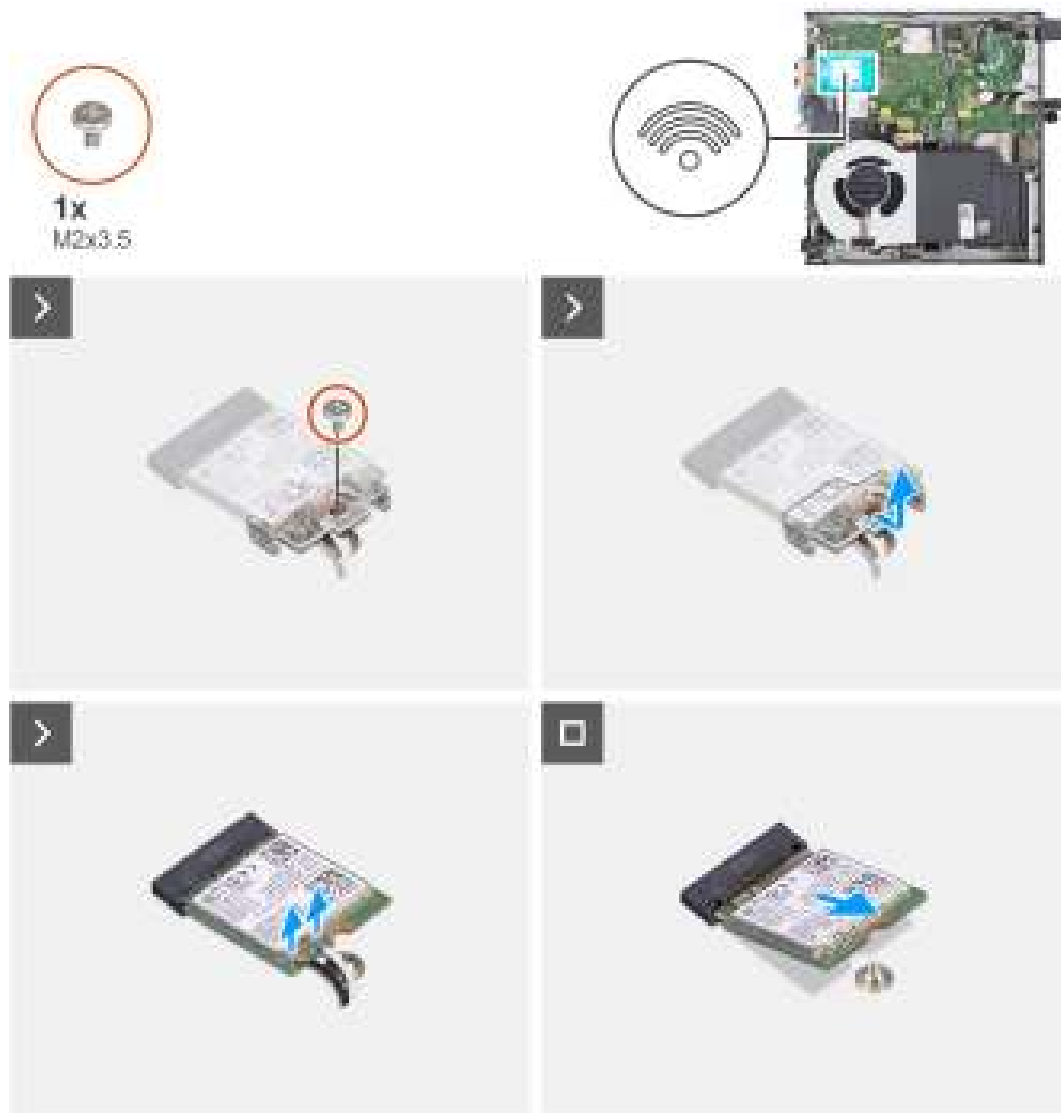
Figure 28. Removing the wireless card
