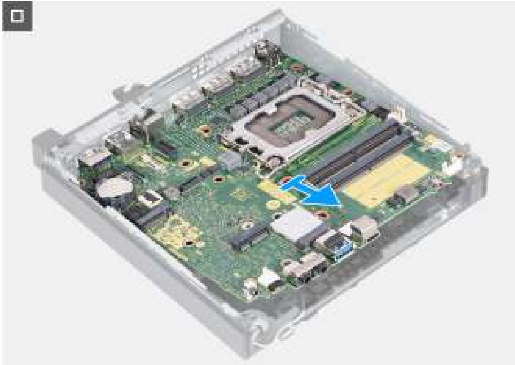
Figure 46. Removing the system board
