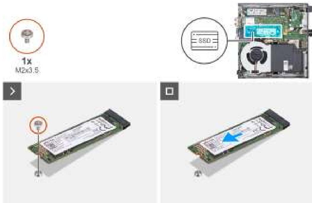
Figure 23. Removing the M.2 2280 solid-state drive from slot 0
