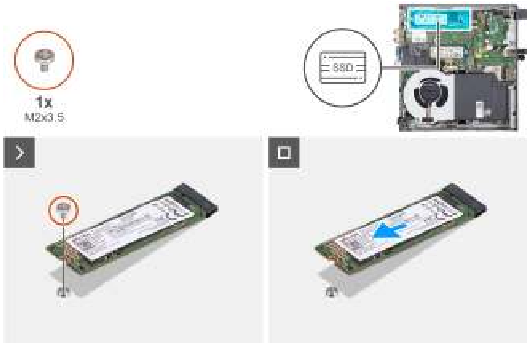
Figure 25. Removing the M.2 2280 solid-state drive from slot 1
