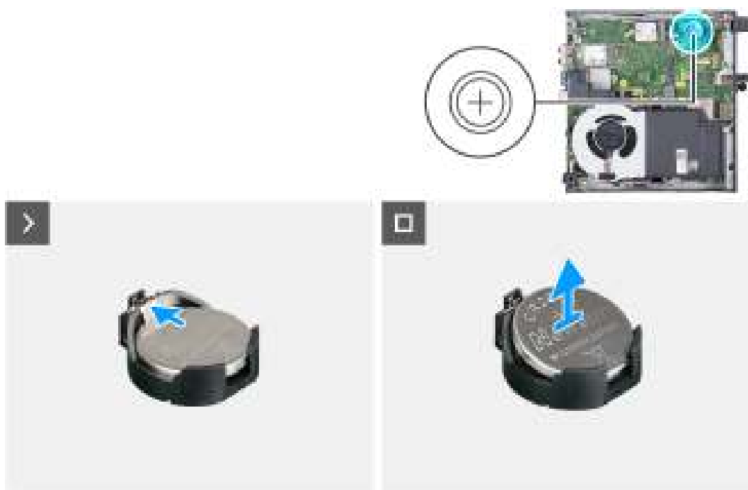
Figure 13. Removing the coin-cell battery
