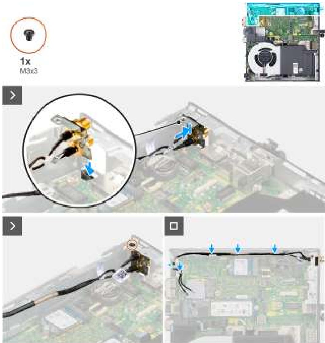
Figure 55. Installing SMA antenna (Location 3)
