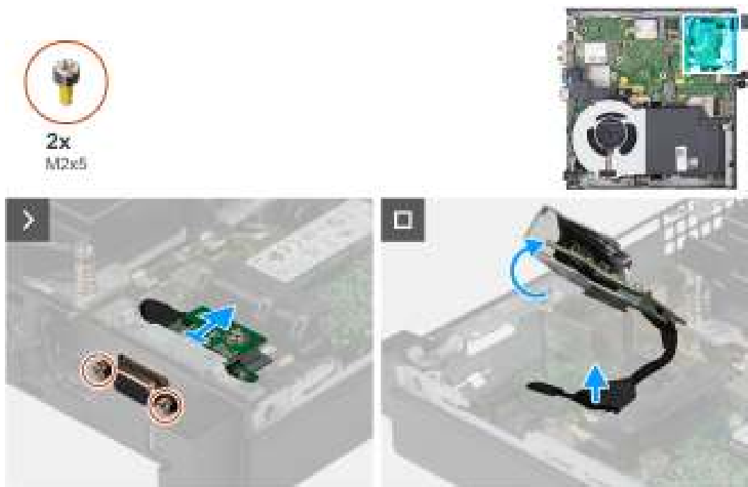
Figure 35. Removing the optional I/O module (VGA or Serial)
