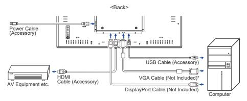
\* VGA cable and Audio cable are not supplied with the monitor. If you use low quality cable, it may cause a result of electro-magnetic interference. Please contact the iiyama Support Centre in your country if you wish to connect the monitor via the VGA cable or Audio cable.
