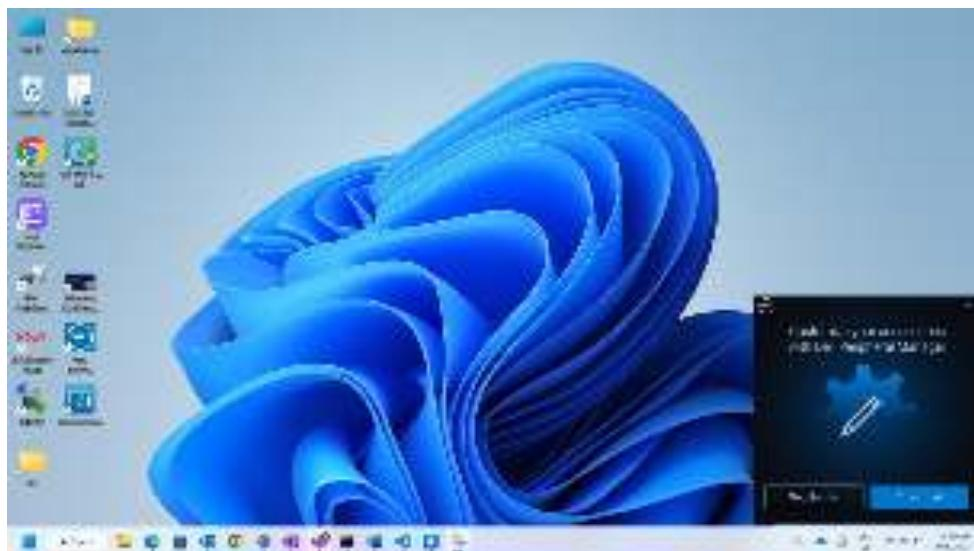
When you connect the device/peripheral to your computer for the first time, a installer prompt is displayed, and you can choose to download Dell Peripheral Manager or to decline the installation.
