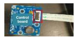
Tear off a black tape from "USB board FFC" and "Panel
