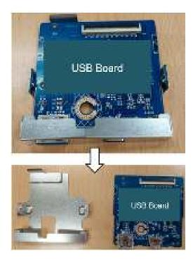
S12 Tear off 2 conductive tapes from "Main Shielding and "Panel"
