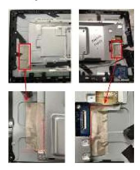
Tear off an aluminum foil and a yellow tape from "LVDS FFC" on "Panel"
