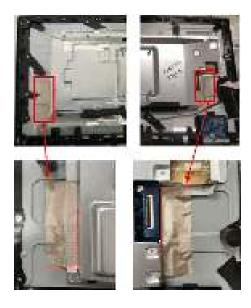
Assemble "USB board" with "USB Shielding"
