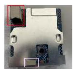
S11 Disassemble "USB board" from "USB Shielding"
