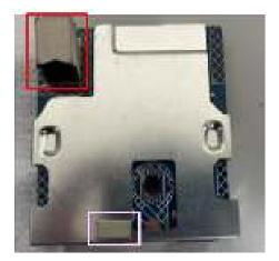
S11 Disassemble "USB board" from "USB Shielding"
