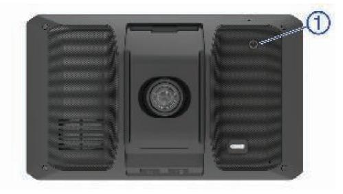
• To put the device in power saving mode, press the power button while the device is on. While in power saving mode, the screen is off and the device uses very little power, but it can wake instantly for use.
