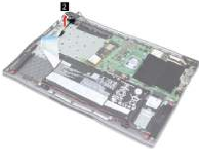
Figure 29. Remove the fingerprint reader module
