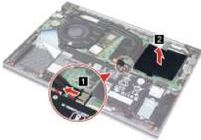
Figure 18. Peel off the memory module mylar
