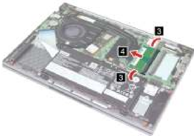
Figure 19. Remove the memory module
