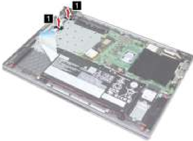
Figure 28. Remove the acetate tapes
