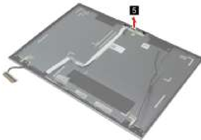
Figure 49. Remove the camera board
