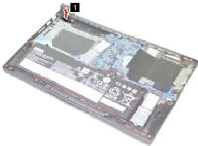
Figure 31. Remove the power button
