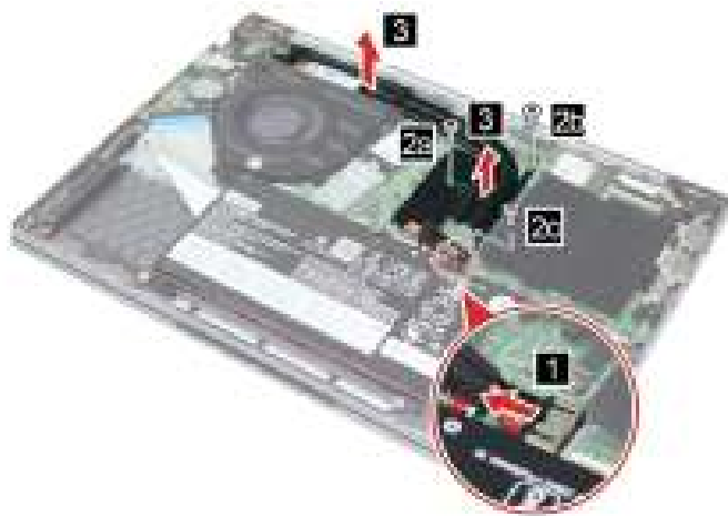
Figure 16. Loosen three screws and remove the heat sink
