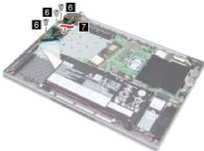
Figure 25. Remove three screws and remove the I/O board with cable
