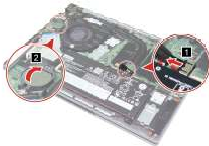
Figure 17. Remove the coin-cell battery
