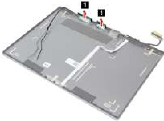
Figure 50. Remove the antennas
