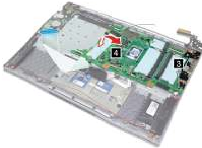
Figure 33. Remove one screw and remove the system board
