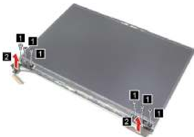
Figure 41. Remove six screws and remove the hinges
