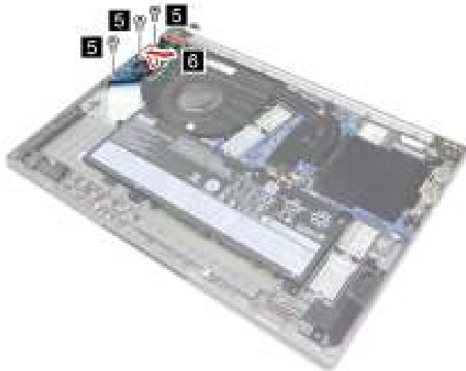
Figure 27. Remove three screws and the I/O board
