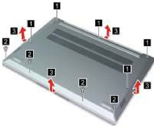
Figure 4. Loosen five screws, remove four screws and the lower case
