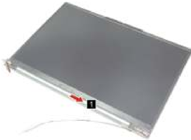
Figure 39. Remove the hinge cover
