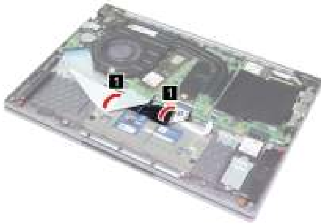
Figure 21. Lift the cables
