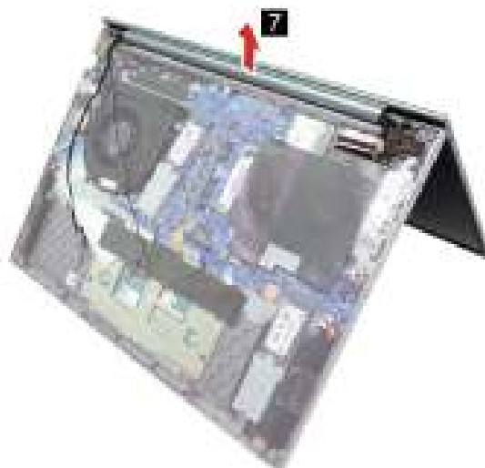
Figure 38. Rotate and remove LCD module
