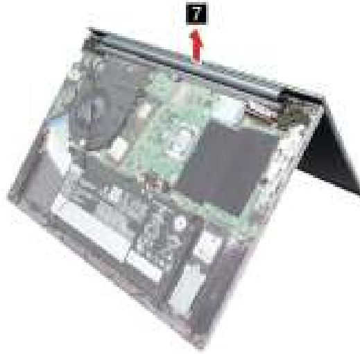
Figure 36. Rotate and remove LCD module
