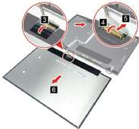
Figure 43. Peel back the camera board cable and EDP cables. Then, remove the LCD panel
