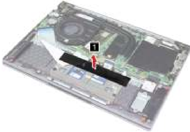
Figure 6. Remove the battery protective sponge
