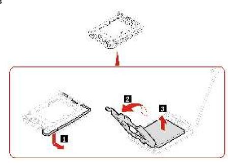
**Note:** Before you attach the microprocessor to the computer, clean all thermal grease that has been used and then apply new thermal grease. Apply new thermal grease at an amount of 0.35 grams, on the parts marked as shown in the following illustrations. Either too much or too less application of grease can cause a thermal problem due to imperfect contact with a component.
