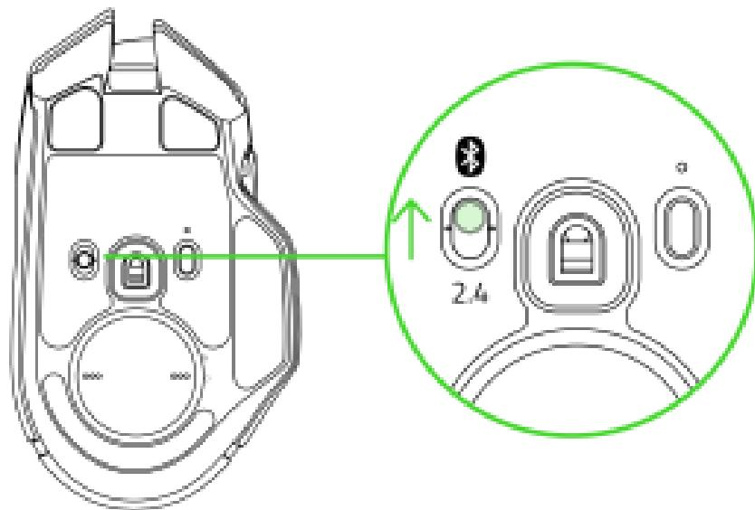
2. Press and hold the scroll wheel, mouse 4, and mouse 5 buttons simultaneously for 3 seconds to activate pairing mode. The scroll wheel and Razer logo will blink twice in repeated intervals to show that the device is in pairing mode.
