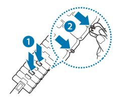
3 Reconnect both sides of the metal band which are disconnected and press the pin to assemble until it clicks. When assembling the pin, be careful for your safety.
