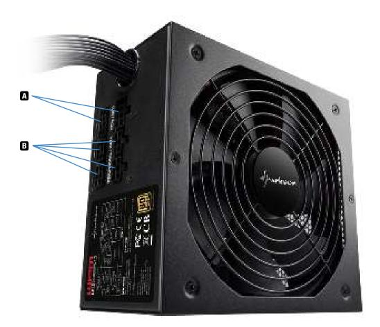
A 2x Sockets for 4+4-Pin CPU Connector\* (CPU) or 6+2-Pin PCIe Connector (PCIe)
