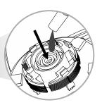
After replacing the fan blades several times, readd the oil into the bearing (about 0.1ml)
