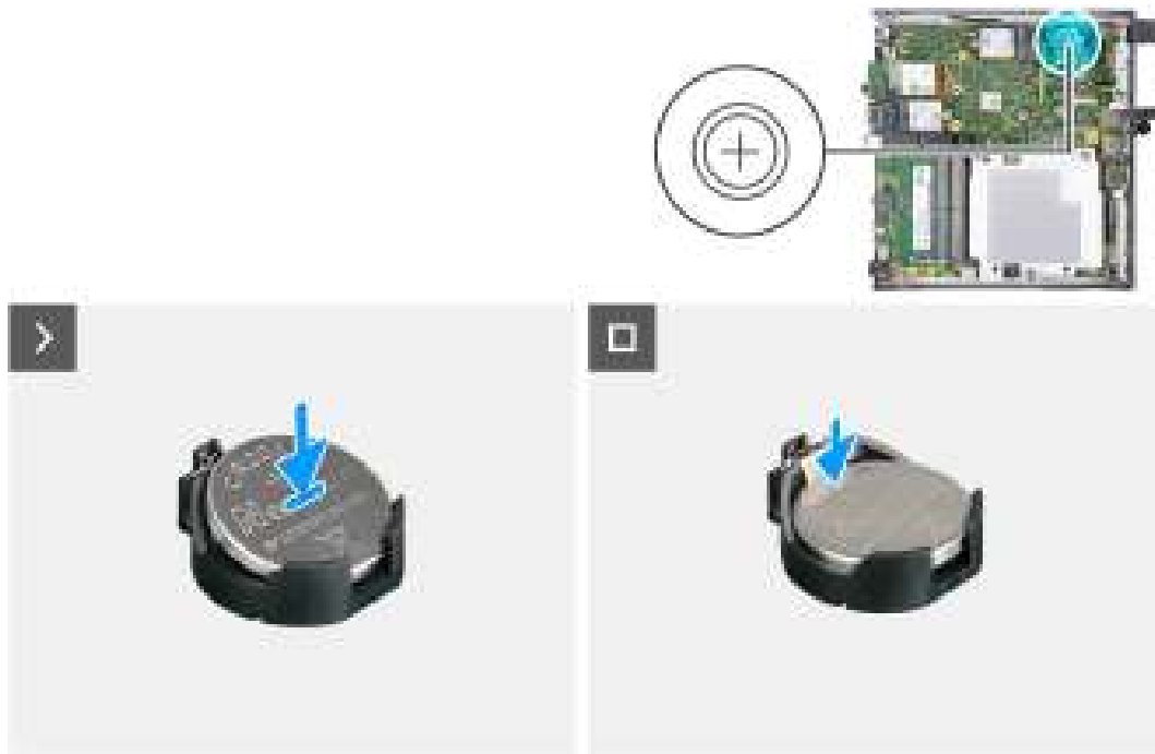
Figure 14. Installation de la pile bouton
