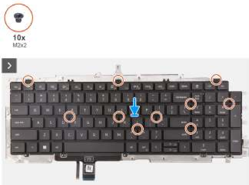
Figure 67. Installation du clavier
