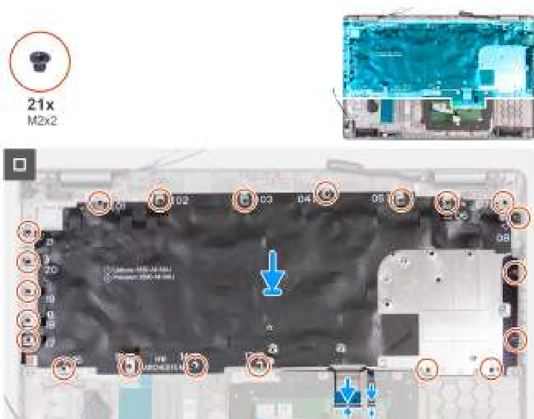
Figure 68. Installation du clavier
